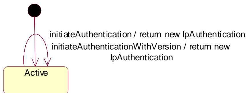
Figure : State Transition Diagram for IpInitial
