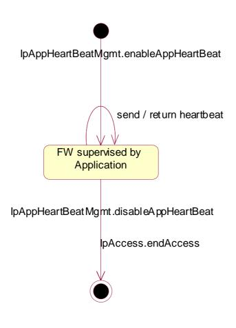
Figure : State Transition Diagram for IpHeatBeat
