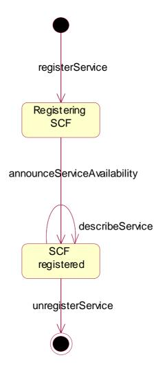
Figure : State Transition Diagram for IpFwServiceRegistration
