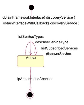
Figure : State Transition Diagram for IpServiceDiscovery
