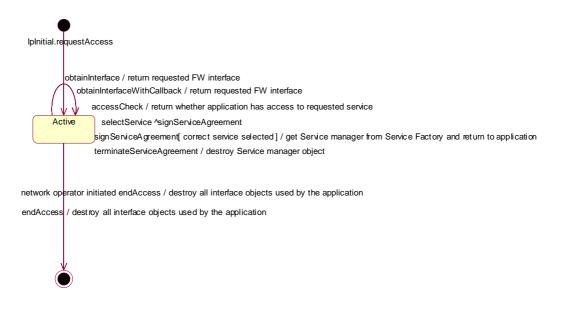
Figure : State Transition Diagram for IpAccess
