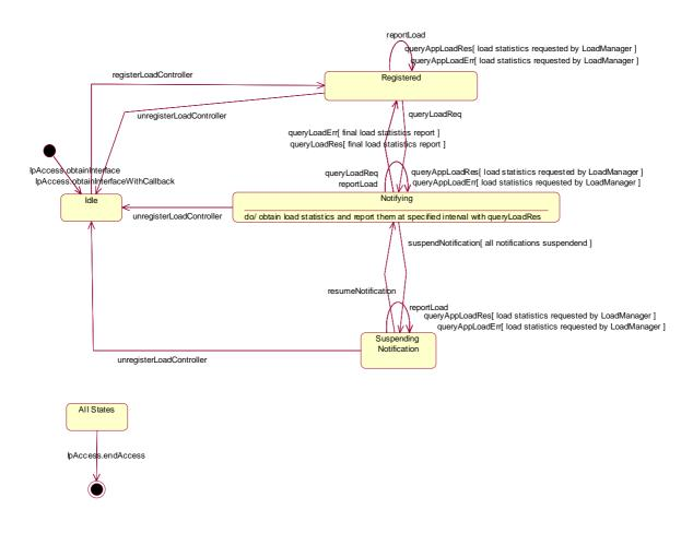
Figure : State Transition Diagram for IpLoadManager
