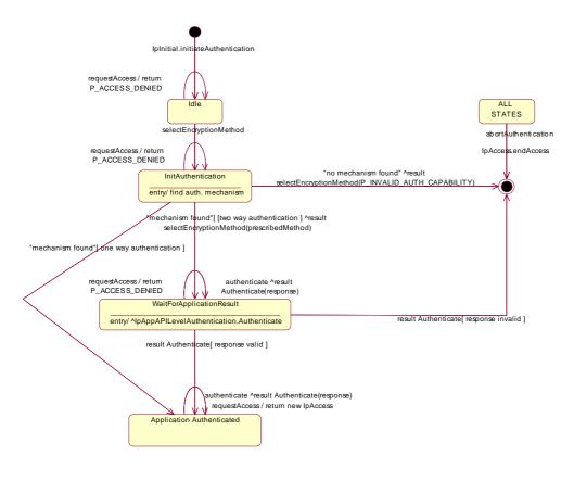
Figure : State Transition Diagram for IpAPILevelAuthentication
