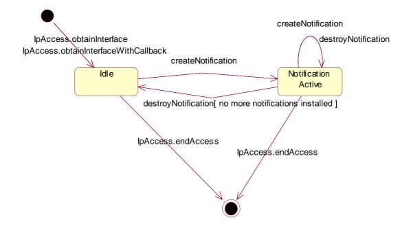
Figure : State Transition Diagram for IpEventNotification
