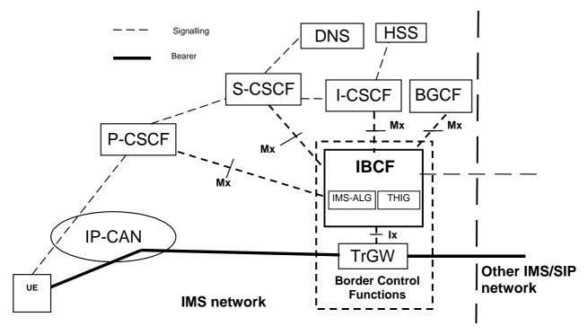
**Figure 3: Border Control Functions**
