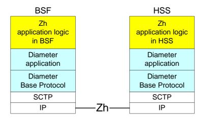
Figure 4.2: Protocol stack of Zh interface
