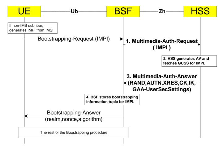
Figure 4.3: The GBA bootstrapping procedure
