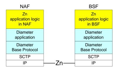
Figure 5.2: Protocol stack of Zn interface
