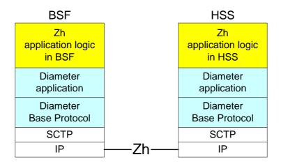
Figure 4.2: Protocol stack of Zh interface
