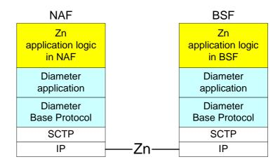
Figure 5.2: Protocol stack of Zn interface
