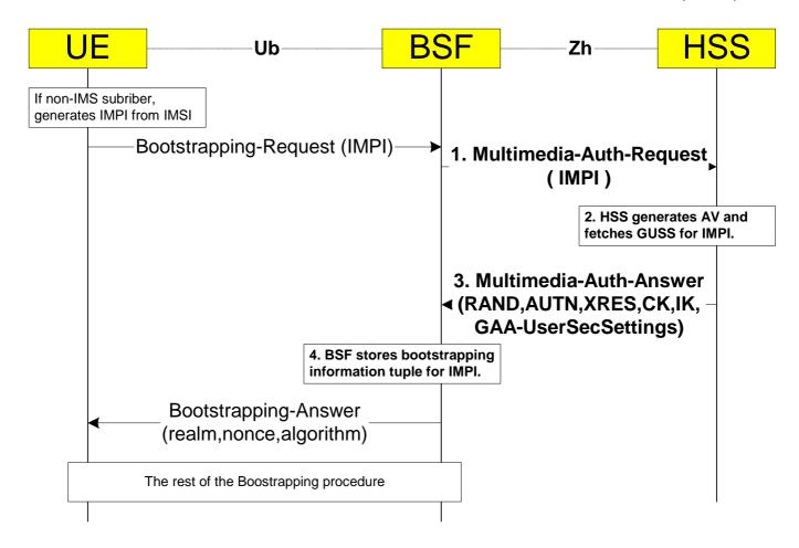
Figure 4.3: The GBA bootstrapping procedure
