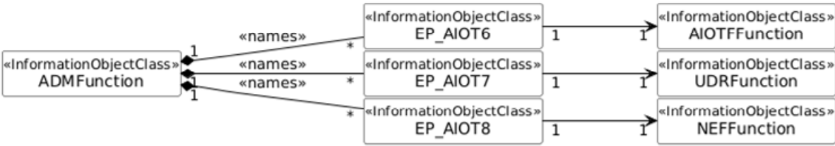
Figure 5.2.1.1-41: Transport view of ADM NRM
