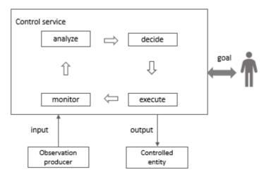
Figure 4.2.4.1.1: Closed control loop entities
