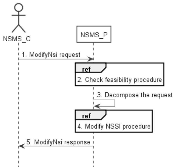
**Figure 7.6-1: Network Slice Instance Modification Request procedure**
