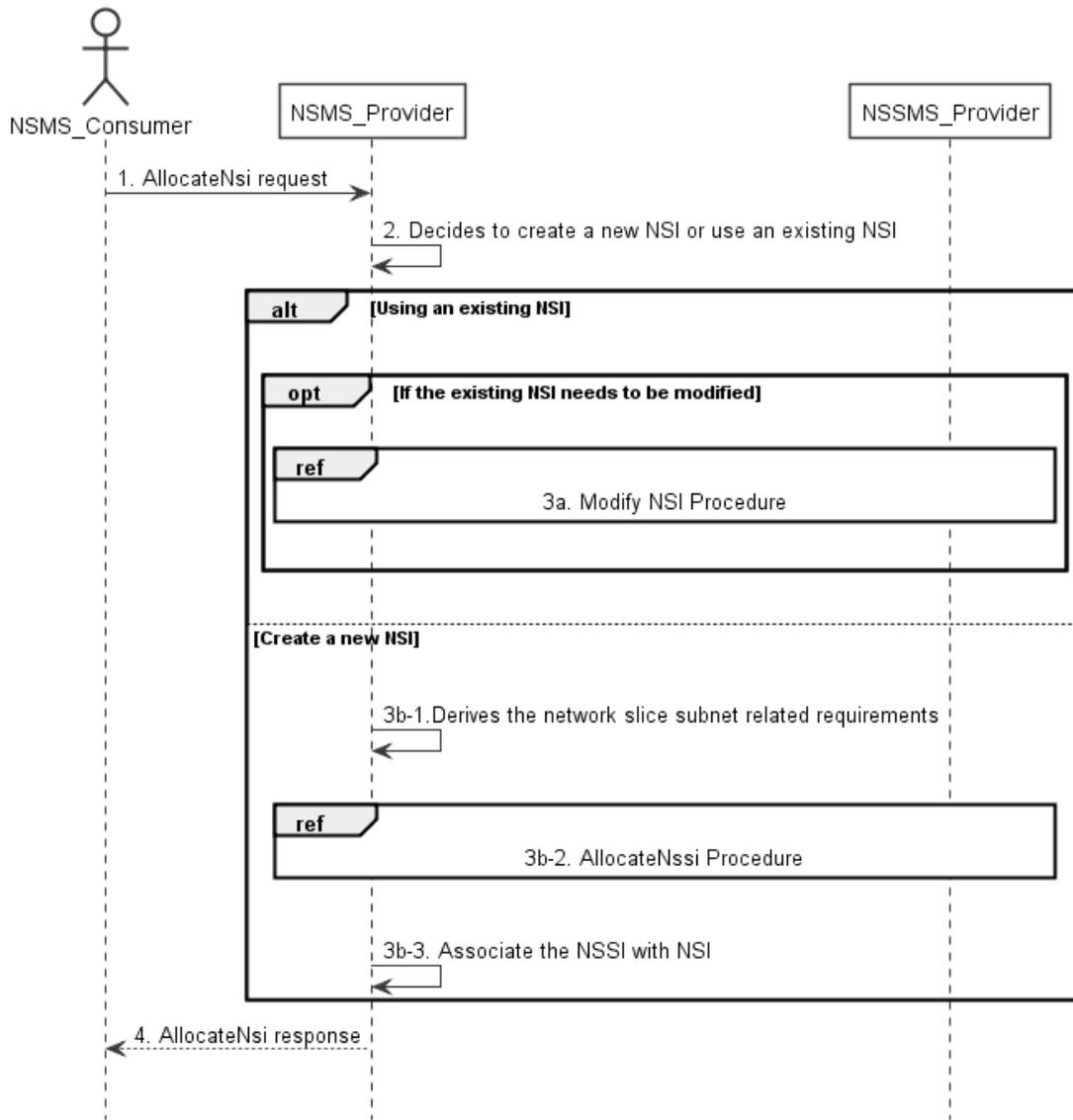
**Figure 7.2-1: Network Slice Instance Allocation Request procedure**
