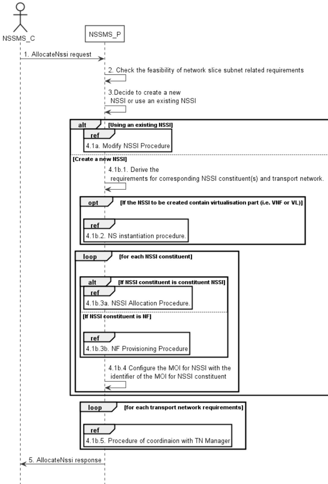
**Figure 7.3-1: Network Slice Subnet Instance Allocation Request procedure**
