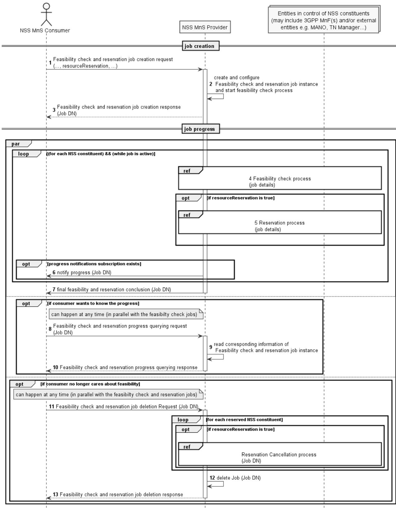
Figure 7.14-2 Network slice subnet feasibility check procedure
