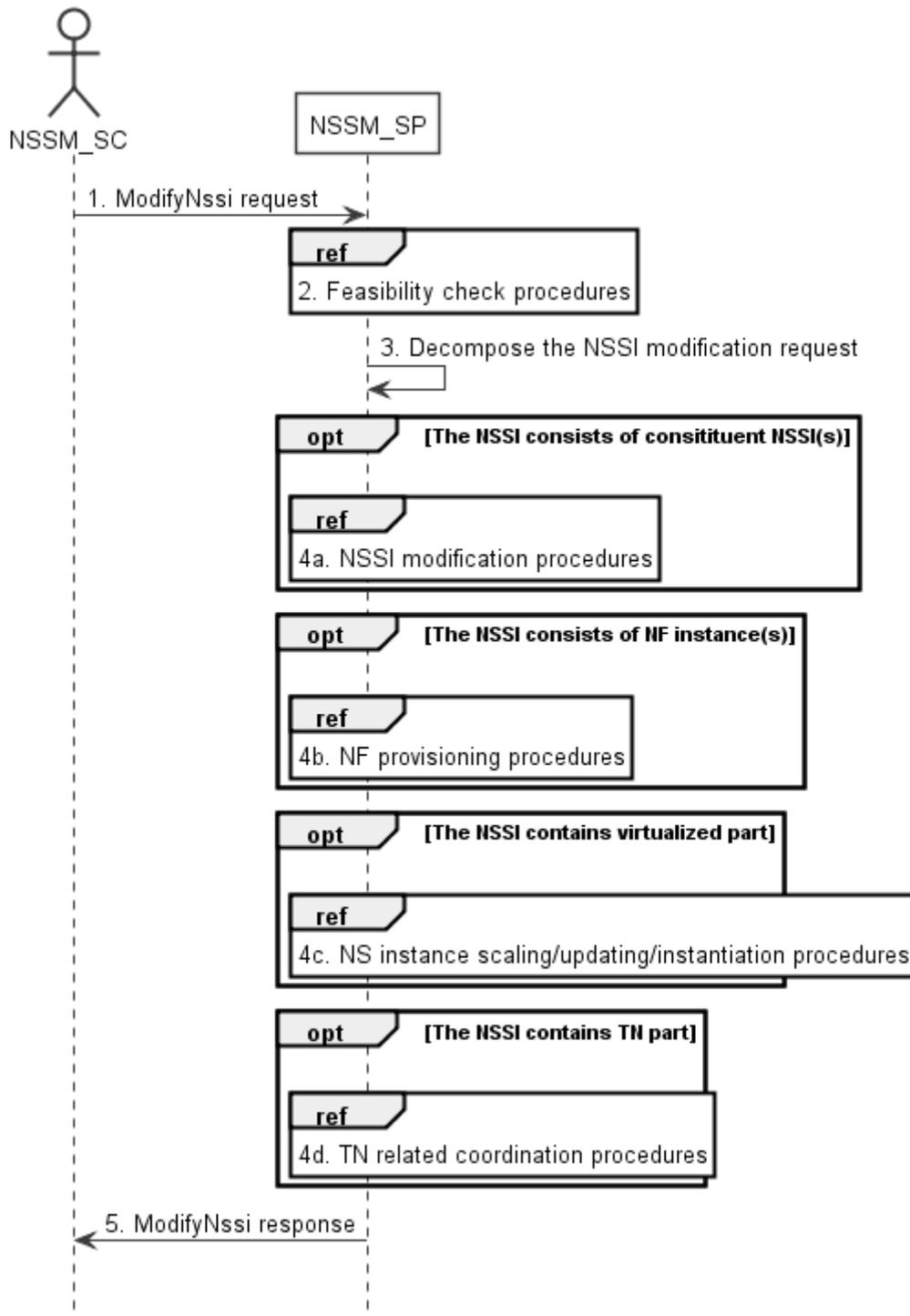
Figure 7.7-1: Network Slice Subnet Instance Modification Request procedure
