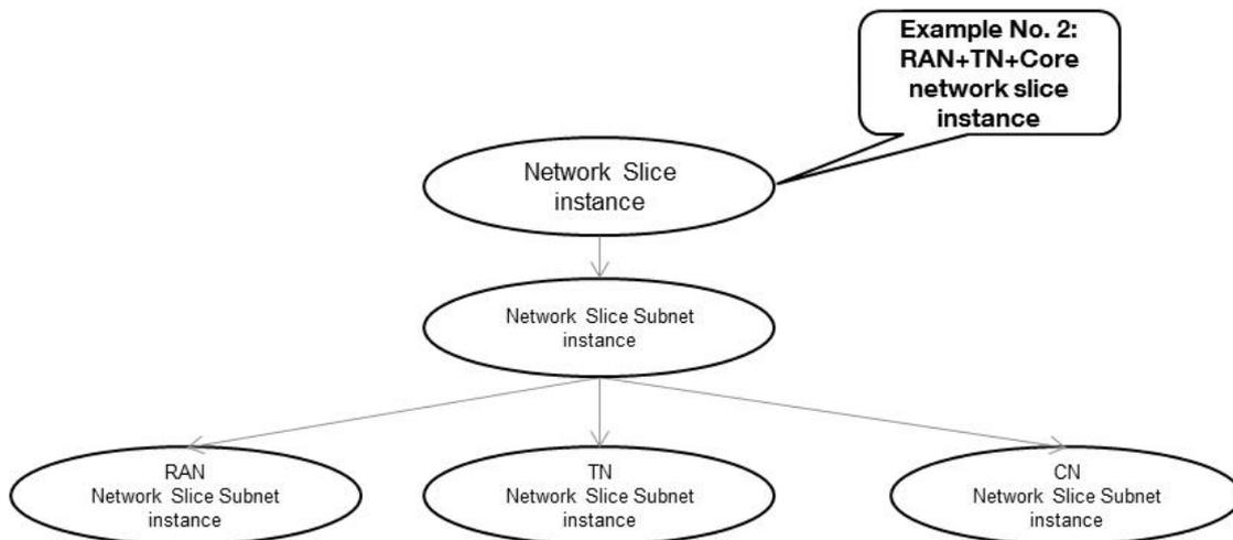
Figure A.4: RAN+TN+CN network slice subnets exposed as network slice
