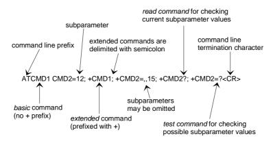
Figure 2: Basic structure of a command line
