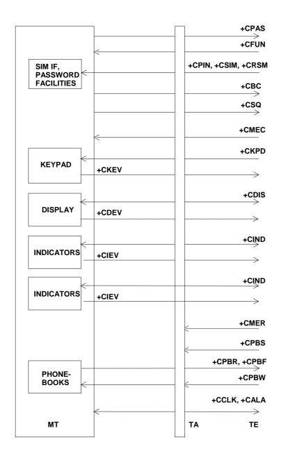
Figure 7: Mobile termination control and status commands
