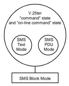
Figure 0.1: Block, Text and PDU modes
