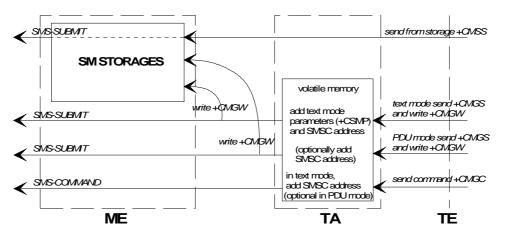
Figure 4: Message service send and write procedures
