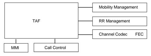
Figure 1: TAF interfacing to other MT functions
