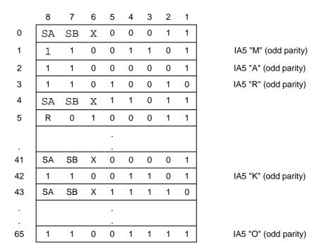
Figure 2c: A 66-octet RLP L2RCOP PDU with status octets separated by more than 23 octets
