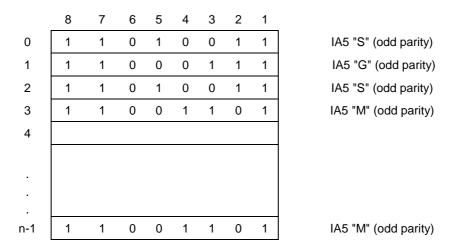
Figure 2b: Multi-link RLP L2RCOP PDU with no status octet transfer
