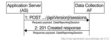
Figure 4.2.5.2-1: Initial configuration of Application Server
