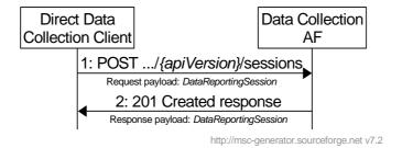
Figure 4.3.2.2-1: Initial configuration of Direct Data Collection Client
