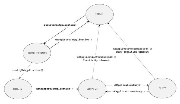
Figure 8.2.1-1: State model diagram
