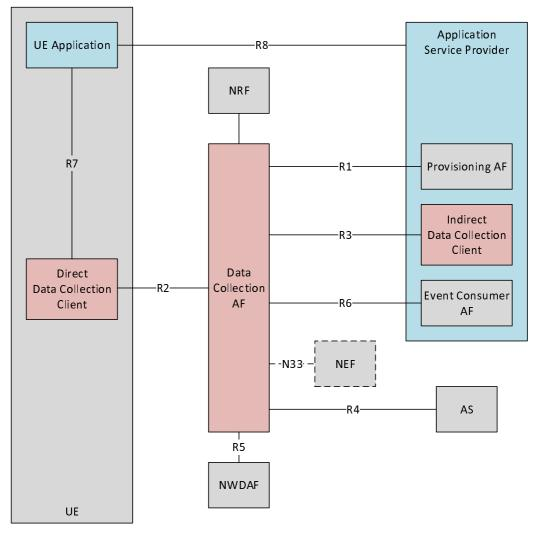
NOTE: The Data Collection AF may be deployed outside the trusted domain, in which case the services it exposes to API invokers are mediated by the NEF. The logical relationships denoted by the reference points are unaffected by such deployment choices.
