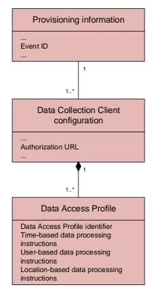
Figure 4.5.2-1: Data exposure restriction domain model
