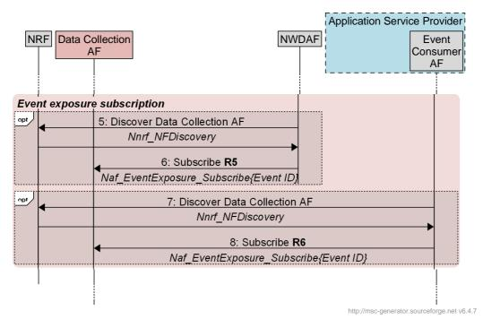
Figure 5.3-1: High-level procedures for subscription phase
