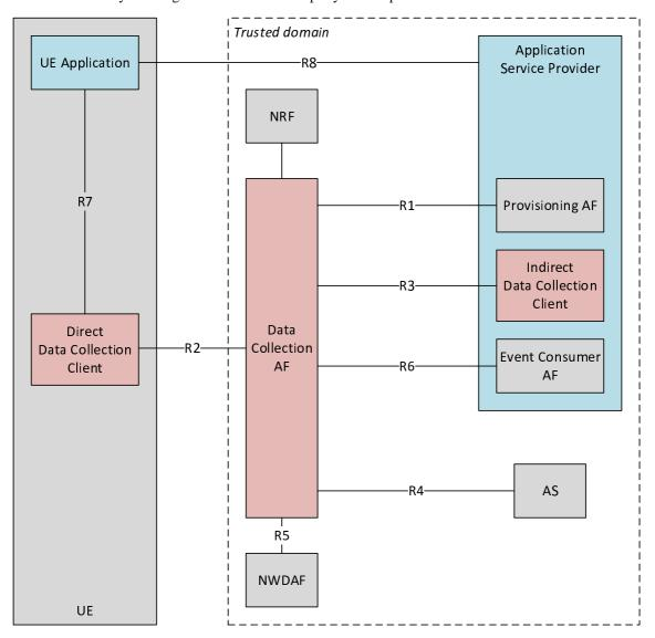
Figure A.2-1: Collaboration A with all functions deployed inside the trusted domain
