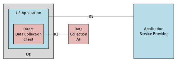
Figure A.6-1: Collaboration E with Data Collection Client deployed as part of the UE Application
