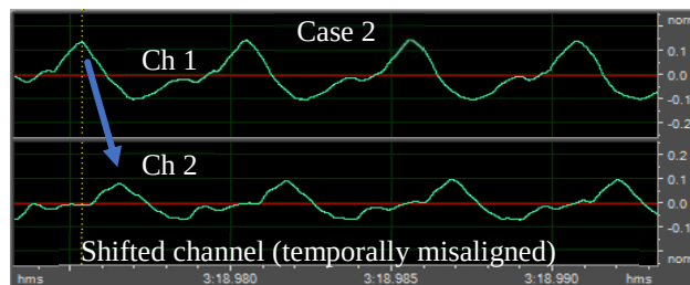
Figure 5.3-10: Temporally Misaligned Audio Signals in Ch1 and Ch2
