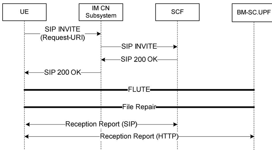
**Figure 31 Procedures for IMS based MBMS Download**
