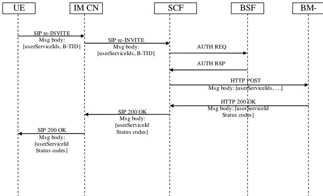
**Figure 24a: SIP based MBMS User Service De-registration**
