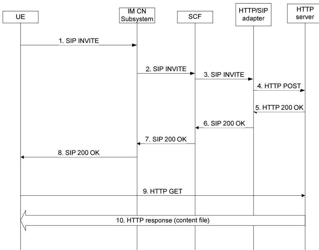
**Figure 33: IMS based session set-up for progressive download**
