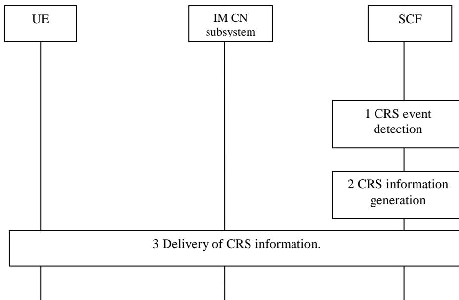
**Figure 47: Procedure for CRS provided by SCF**
