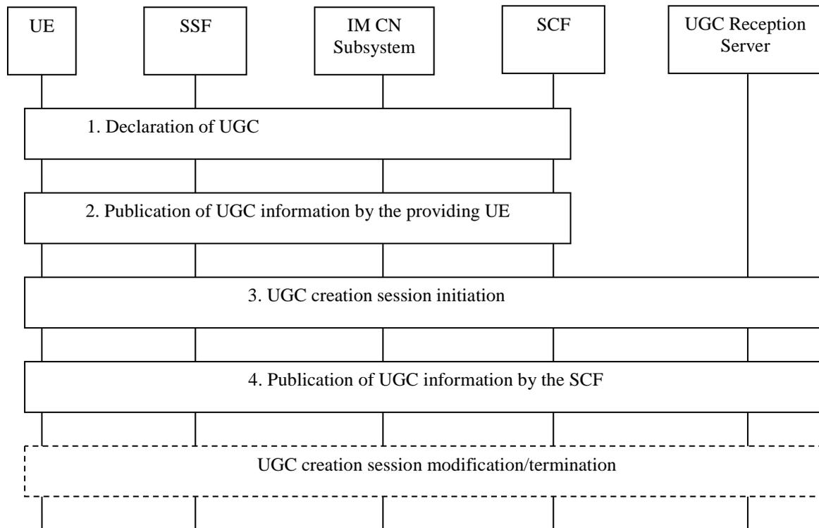
**Figure 30 : IMS Based UGC Provision Procedures**
