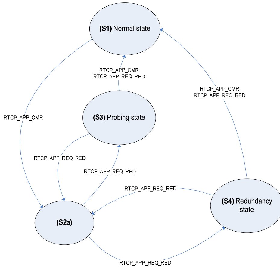
Figure C.3: State diagram for simplified four-state adaptation state machine
