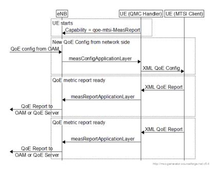
Figure L-2: Example signalling diagram for LTE
