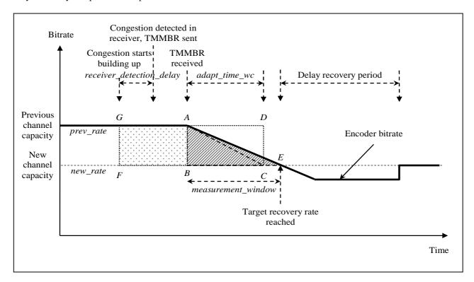
Figure C.8. Schematic figure of bitrate reduction in video encoder when the encoder cannot immediately switch to the requested bitrate
