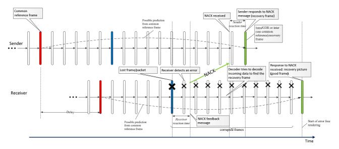
Figure P.1 Video error recovery using NACK feedback message.
