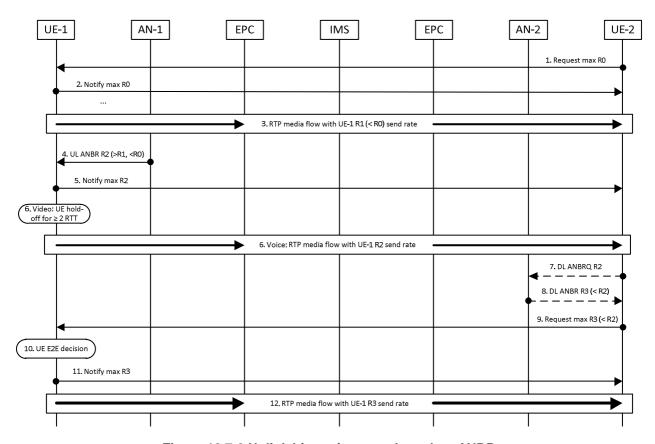
Figure 10.7-2 Uplink bitrate increase based on ANBR
