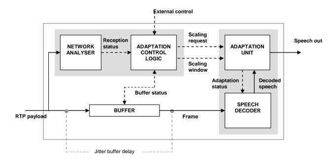
Figure 8.1: Example structure of an MTSI speech receiver
