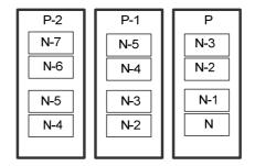
Figure 10.12: Payload packetization with 100 % redundancy and 2 frames aggregated per packet
