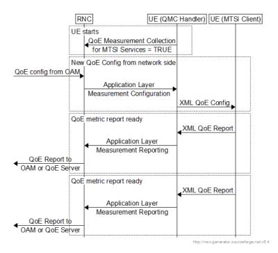
Figure L-1: Example signalling diagram for UMTS
