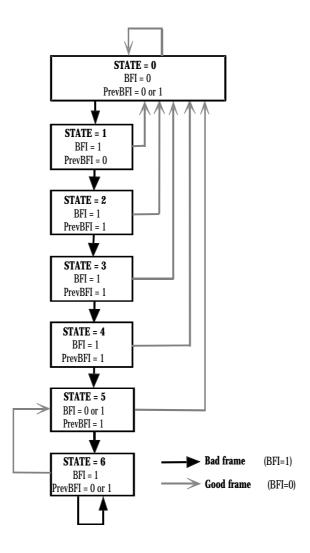
Figure 1: State machine for controlling the bad frame substitution
