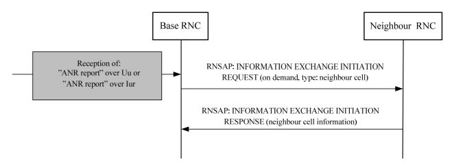
Figure 5.2.2-1 Neighbour Cell Configuration using lur
