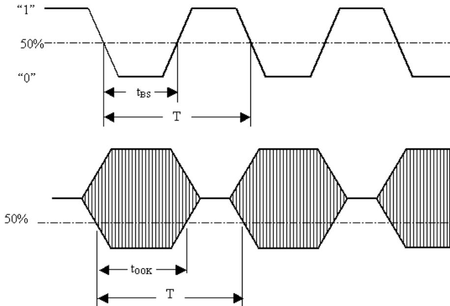
Duty cycle for bit stream =  $t_{BS}/T$ ; duty cycle for OOK =  $T_{OOK}/T$
