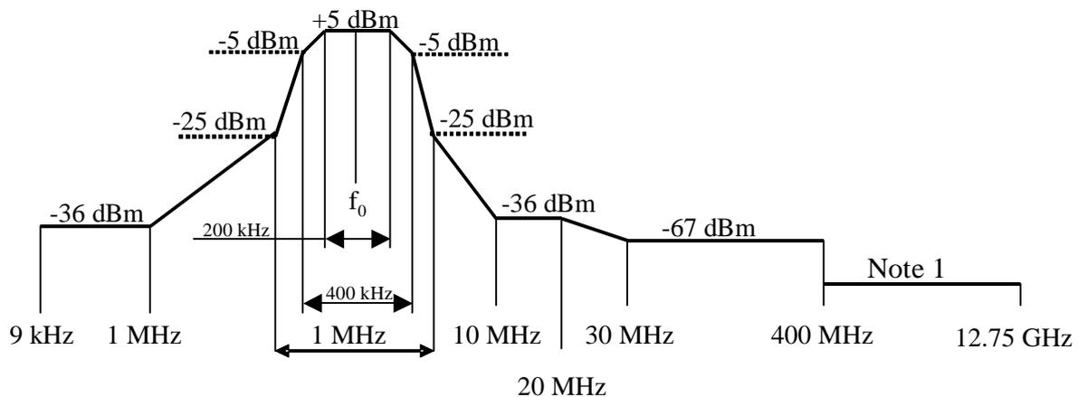
Figure 4.3.4.2.1: Modem spectrum emission mask.
