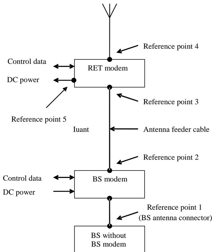
Figure 4.3.1: Modem configuration and modem reference points for a BS without BS modem
