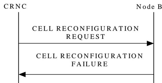
**Figure 19: Cell Reconfiguration procedure: Unsuccessful Operation**
