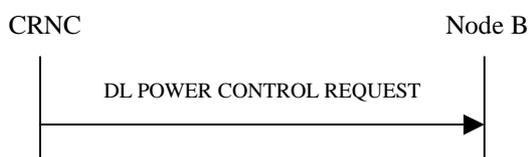
**Figure 37: Downlink Power Control procedure, Successful Operation**
