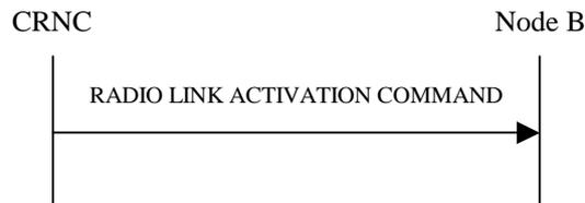
**Figure 47D: Radio Link Activation procedure**
