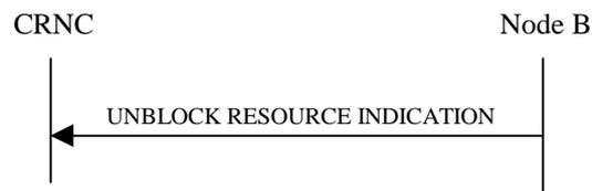
**Figure 8: Unblock Resource procedure, Successful Operation**
