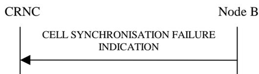
**Figure 27I Cell Synchronisation Failure procedure, Successful Operation**
