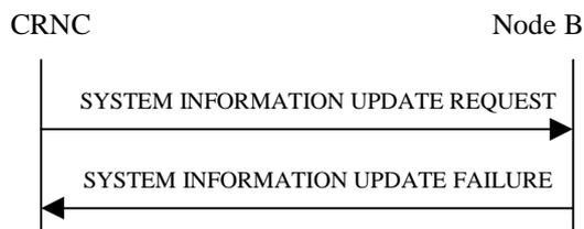
**Figure 23: System Information Update procedure, Unsuccessful Operation**
