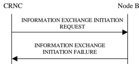
**Figure 27M: Information Exchange Initiation procedure, Unsuccessful Operation**
