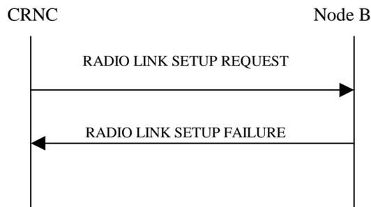
**Figure 25: Radio Link Setup procedure, Unsuccessful Operation**
