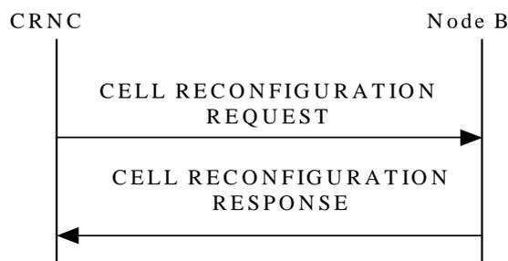
**Figure 18: Cell Reconfiguration procedure, Successful Operation**
