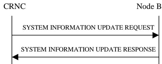
**Figure 22: System Information Update procedure, Successful Operation**
