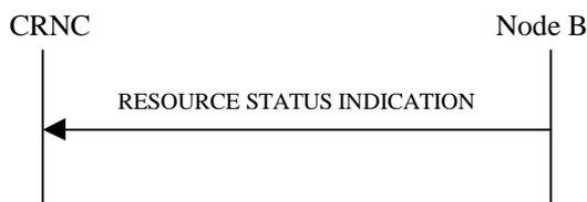
**Figure 21: Resource Status Indication procedure, Successful Operation**
