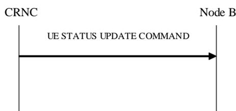
**Figure 27R: UE Status Update procedure, Successful Operation**
