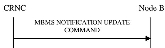
**Figure 27Q: MBMS Notification Update procedure, Successful Operation**
