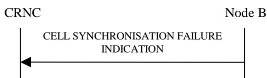
**Figure 271 Cell Synchronisation Failure procedure, Successful Operation**
