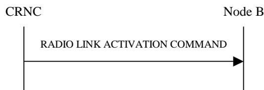
**Figure 47D: Radio Link Activation procedure**
