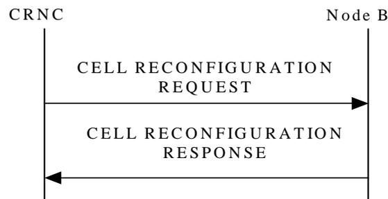
**Figure 18: Cell Reconfiguration procedure, Successful Operation**
