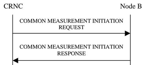
**Figure 11: Common Measurement Initiation procedure, Successful Operation**
