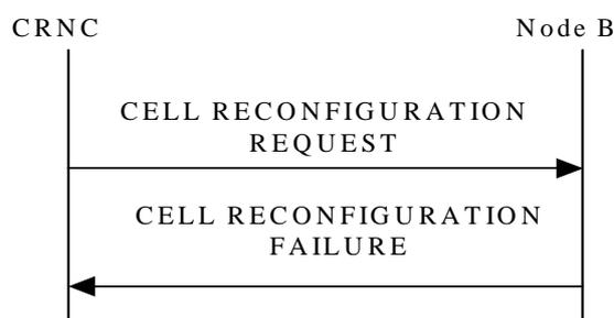
**Figure 19: Cell Reconfiguration procedure: Unsuccessful Operation**
