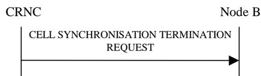
**Figure 27H Cell Synchronisation Termination procedure, Successful Operation**
