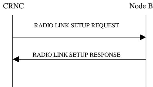
**Figure 24: Radio Link Setup procedure, Successful Operation**
