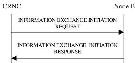
**Figure 27L: Information Exchange Initiation procedure, Successful Operation**
