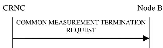
**Figure 14: Common Measurement Termination procedure, Successful Operation**
