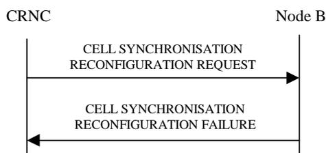
**Figure 27F Cell Synchronisation Reconfiguration procedure, Unsuccessful Operation**
