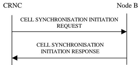
**Figure 27C Cell Synchronisation Initiation procedure, Successful Operation**
