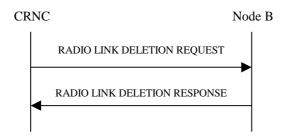
Figure 36: Radio Link Deletion procedure, Successful Operation
