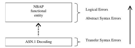
Figure 38: Protocol Errors in NBAP.
