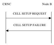
Figure 17: Cell Setup procedure: Unsuccessful Operation
