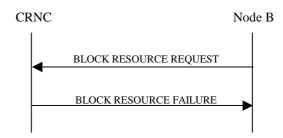
Figure 7: Block Resource procedure, Unsuccessful Operation
