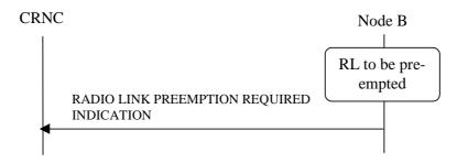
Figure 47B: Radio Link Pre-emption procedure, Successful Operation
