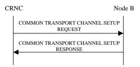
Figure 1: Common Transport Channel Setup procedure, Successful Operation
