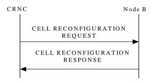
Figure 18: Cell Reconfiguration procedure, Successful Operation
