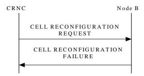
Figure 19: Cell Reconfiguration procedure: Unsuccessful Operation
