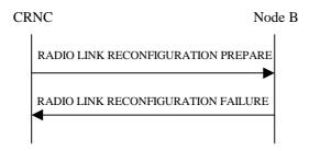
Figure 31: Synchronised Radio Link Reconfiguration Preparation procedure, Unsuccessful Operation
