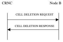
Figure 20: Cell Deletion procedure, Successful Operation
