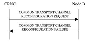
Figure 4: Common Transport Channel Reconfiguration procedure, Unsuccessful Operation
