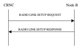
Figure 24: Radio Link Setup procedure, Successful Operation
