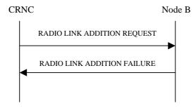
Figure 29: Radio Link Addition procedure: Unsuccessful Operation
