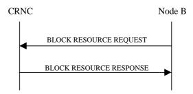
Figure 6: Block Resource procedure, Successful Operation
