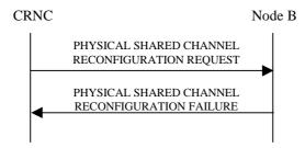
Figure 27: Physical Shared Channel Reconfiguration procedure: Unsuccessful Opreration
