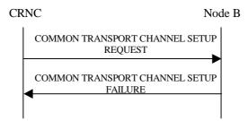
Figure 2: Common Transport Channel Setup procedure, Unsuccessful Operation
