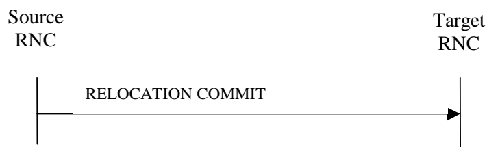
Figure 3: Relocation Commit procedure, Successful Operation
