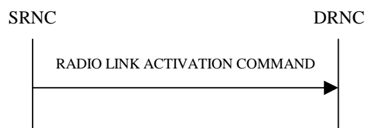
Figure 26D: Radio Link Activation procedure
