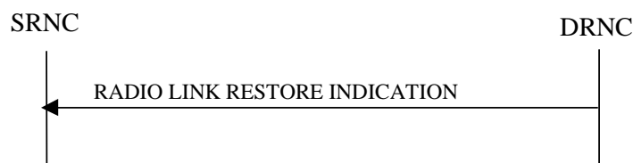
Figure 19: Radio Link Restoration procedure, Successful Operation
