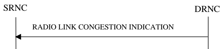
Figure 26C: Radio Link Congestion procedure, Successful Operation
