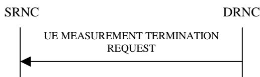
Figure 261: UE Measurement Termination procedure, Successful Operation
