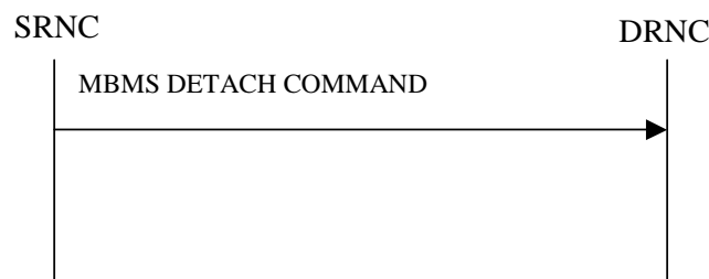
Figure 32: MBMS Detach procedure, Successful Operation
