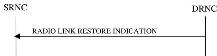
Figure 19: Radio Link Restoration procedure, Successful Operation
