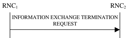
Figure 30I: Information Exchange Termination procedure, Successful Operation
