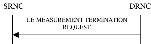
Figure 26I: UE Measurement Termination procedure, Successful Operation
