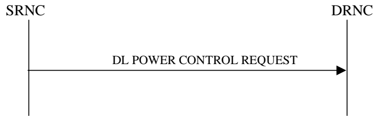
Figure 25: Downlink Power Control procedure, Successful Operation
