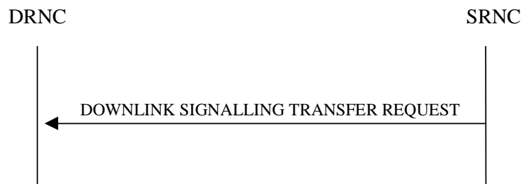
Figure 2: Downlink Signalling Transfer procedure, Successful Operation
