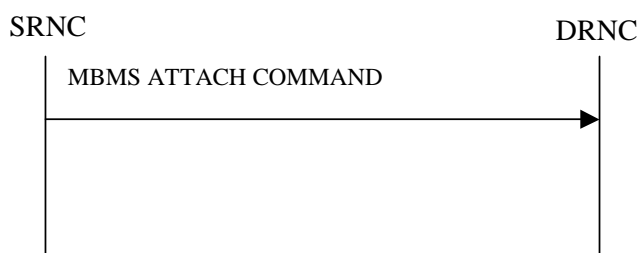
Figure 31: MBMS Attach procedure, Successful Operation
