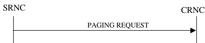
Figure 4: Paging procedure, Successful Operation
