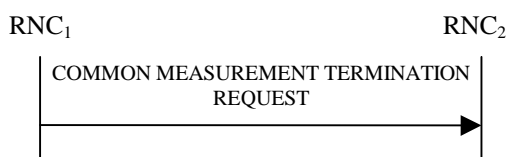
Figure 30D: Common Measurement Termination procedure, Successful Operation
