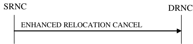
Figure 26O: Enhanced Relocation Cancel procedure: Successful Operation
