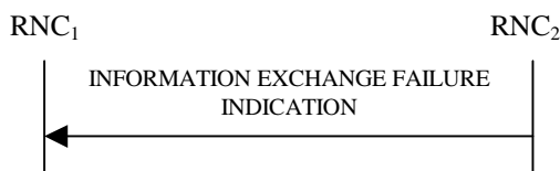
Figure 30J: Information Exchange Failure procedure, Successful Operation
