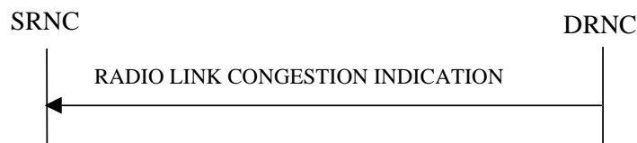
Figure 26C: Radio Link Congestion procedure, Successful Operation
