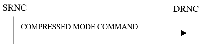
Figure 26: Compressed Mode Command procedure, Successful Operation
