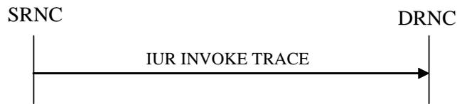
**Figure 26K: Iur Invoke Trace procedure, Successful Operation**
