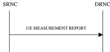
**Figure 26H: UE Measurement Reporting procedure, Successful Operation**
