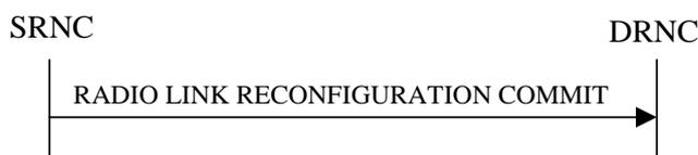
**Figure 12: Synchronised Radio Link Reconfiguration Commit procedure, Successful Operation**
