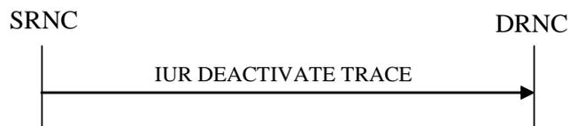
**Figure 26L: Iur Deactivate Trace procedure, Successful Operation**
