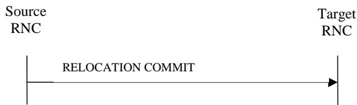
**Figure 3: Relocation Commit procedure, Successful Operation**
