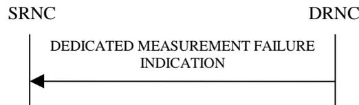
**Figure 24: Dedicated Measurement Failure procedure, Successful Operation**
