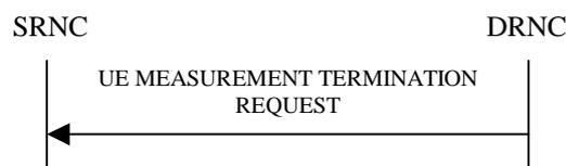
**Figure 26I: UE Measurement Termination procedure, Successful Operation**
