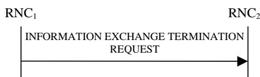
**Figure 30I: Information Exchange Termination procedure, Successful Operation**
