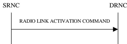
**Figure 26D: Radio Link Activation procedure**
