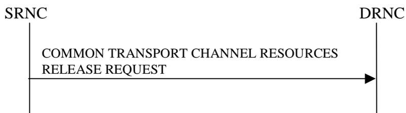
**Figure 29: Common Transport Channel Resources Release procedure, Successful Operation**
