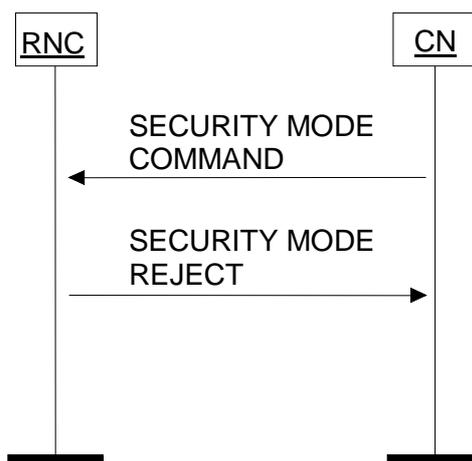
**Figure 20: Security Mode Control procedure. Unsuccessful operation.**
