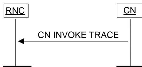
Figure 18: CN Invoke Trace procedure. Successful operation.
