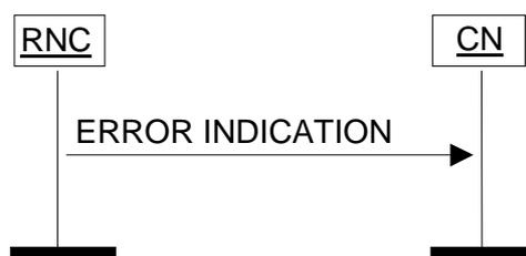
**Figure 32: Error Indication procedure, RNC originated. Successful operation.**
