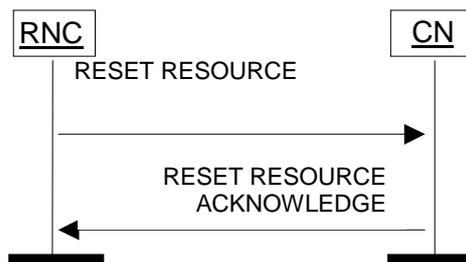
**Figure 34: RNC initiated Reset Resource procedure. Successful operation.**
