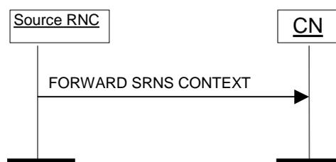
**Figure 14: SRNS Context forwarding from source RNC to CN. Successful operation.**
