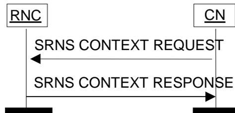
**Figure 12: SRNS Context Transfer procedure. Successful operation.**
