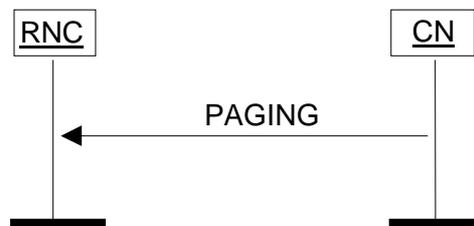
**Figure 16: Paging procedure. Successful operation.**
