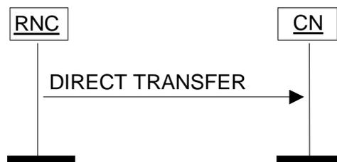
**Figure 26: Direct Transfer, RNC originated. Successful operation.**
