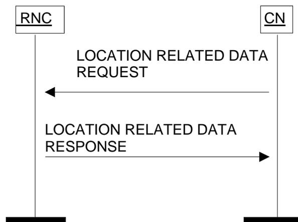
**Figure 37: Location Related Data procedure. Successful operation.**
