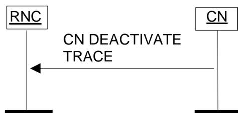
**Figure 33: CN Deactivate Trace procedure. Successful operation.**
