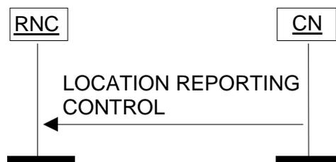
**Figure 21: Location Reporting Control procedure. Successful operation.**
