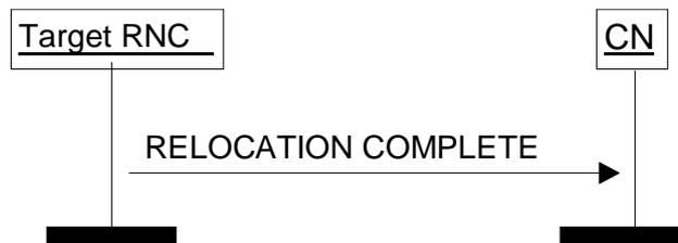
**Figure 10: Relocation Complete procedure. Successful operation.**
