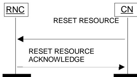
**Figure 35: CN initiated Reset Resource procedure. Successful operation.**
