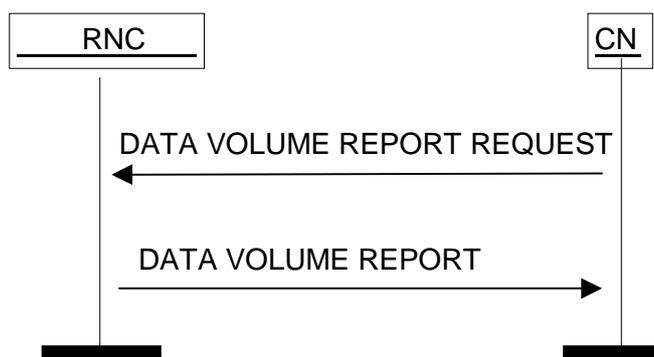
**Figure 23: Data Volume Report procedure. Successful operation.**
