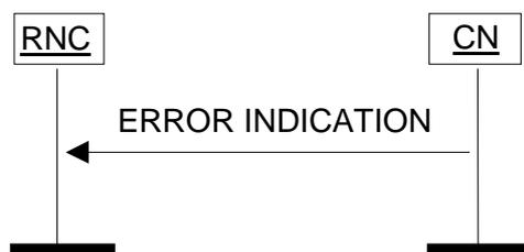
Figure 31: Error Indication procedure, CN originated. Successful operation.
