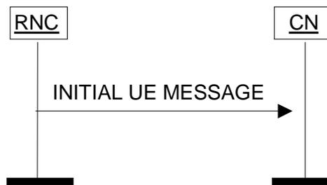
**Figure 24: Initial UE Message procedure. Successful operation.**
