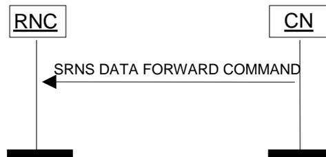
**Figure 13: SRNS Data Forwarding Initiation procedure. Successful operation.**
