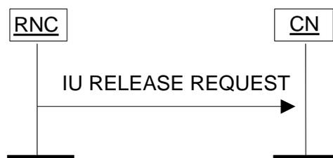
**Figure 3: Iu Release Request procedure. Successful operation.**
