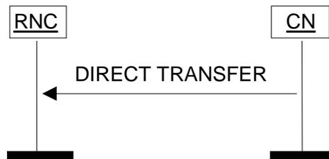
**Figure 25: Direct Transfer, CN originated. Successful operation.**
