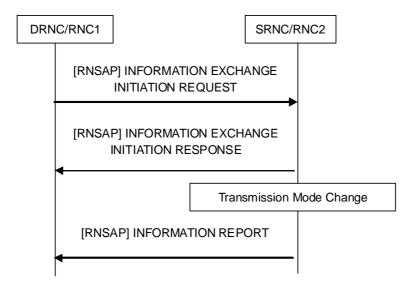
Figure 8.2.13: Information Exchange Initiation signalling flow: Successful Operation.
