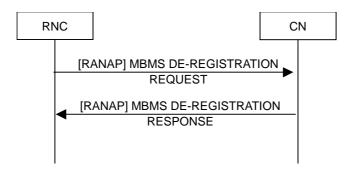
Figure 8.2.5: RNC MBMS De-Registration procedure.
