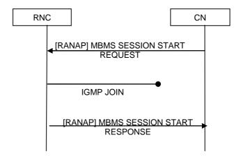
Figure 8.2.16-1: MBMS Session Start procedure. Successful operation.
