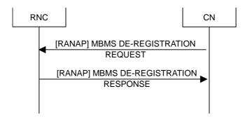
Figure 8.2.6: CN MBMS De-Registration procedure.
