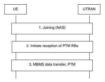
Figure 8.1.2: Joining with continuation of p-t-m
