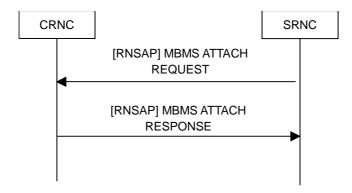
Figure 8.2.11-1: MBMS attach request signalling flow: Successful Operation.
