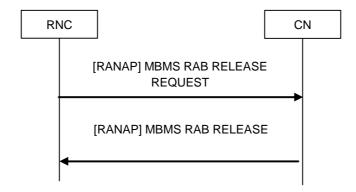
Figure 8.2.15: MBMS RAB Release Request procedure.
