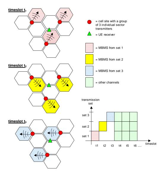
Figure 7.1.bis: Example of non-time-coincident macro diversity transmission
