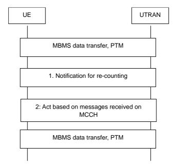
Figure 8.1.3: Recounting with continuation of p-t-m
