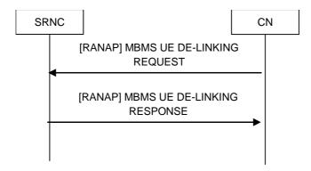
Figure 8.2.9: MBMS UE De-linking signalling flow
