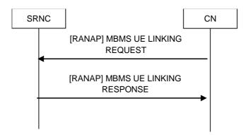
Figure 8.2.8: MBMS UE linking signalling flow
