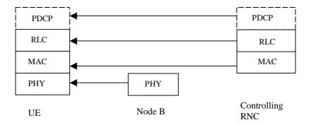
Figure 5.3.1-1: Protocol Stack for MTCH
