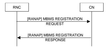
Figure 8.2.4: MBMS Registration procedure.
