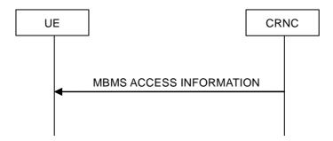
Figure 8.3.4: MBMS Access Information signalling flow
