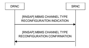
Figure 8.2.12: Channel Type Reconfiguration signalling flow: Successful Operation.
