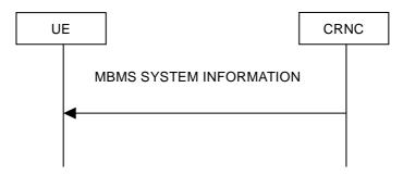
Figure 8.3.1: Broadcast of MBMS system information.
