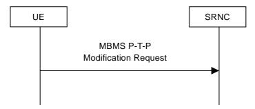
Figure 8.3.9: MBMS P-T-P Modification Request.
