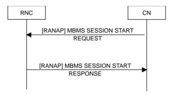
Figure 8.2.1: MBMS Session Start procedure. Successful operation.
