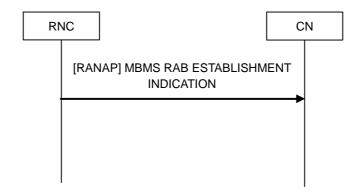
Figure 8.2.14: MBMS RAB Establishment Indication procedure
