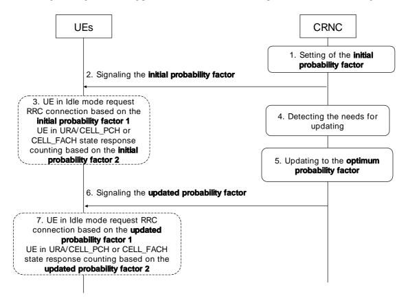
Figure 11.1: MBMS Access Control Procedure
