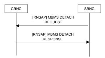
Figure 8.2.11-2: MBMS detach request signalling flow: Successful Operation.
