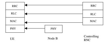
Figure 5.3.2-1: Protocol Stack for MCCH and MSCH
