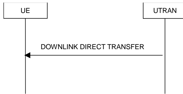
Figure 8.1.9-1: Downlink Direct transfer, normal flow
