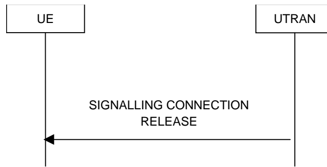
Figure 8.1.13-1: Signalling connection release procedure, normal case
