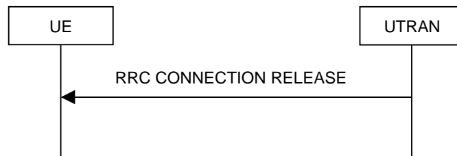
Figure 8.1.4-2: RRC Connection Release procedure on the CCCH
