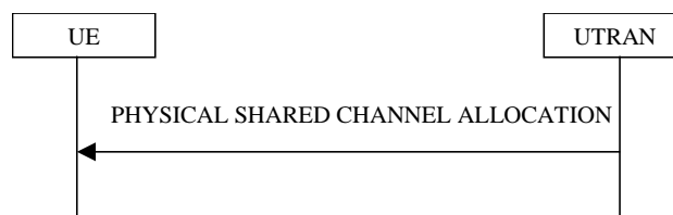
Figure 8.2.7-1: Physical Shared Channel Allocation
