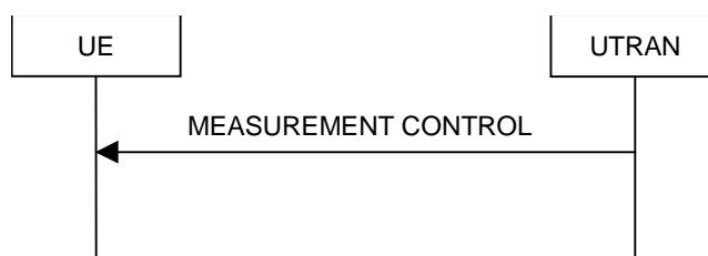
Figure 8.4.1-1: Measurement Control, normal case
