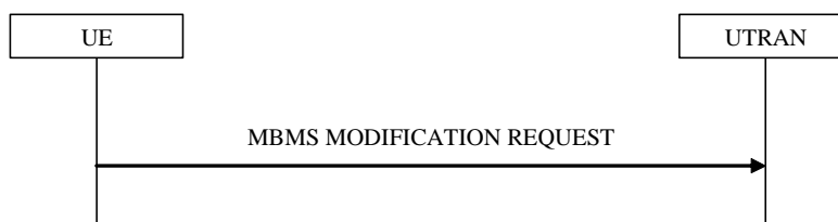
Figure 8.7.6-1: MBMS modification request, normal
