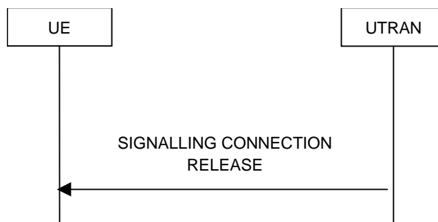
Figure 8.1.13-1: Signalling connection release procedure, normal case
