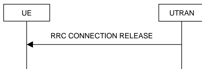
Figure 8.1.4-2: RRC Connection Release procedure on the CCCH
