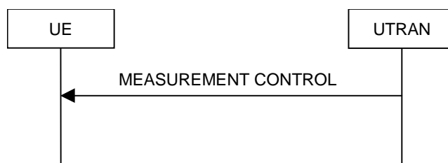
Figure 8.4.1-1: Measurement Control, normal case
