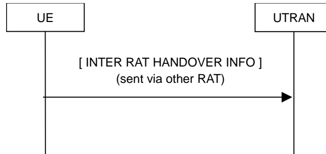
Figure 8.1.16-1: Inter RAT handover information transfer, normal flow
