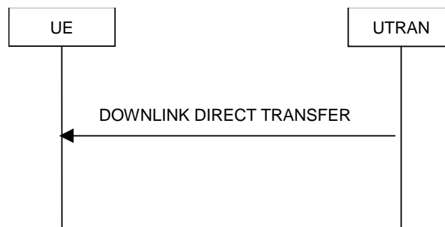
Figure 8.1.9-1: Downlink Direct transfer, normal flow
