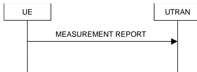
Figure 8.4.2-1: Measurement report, normal case
