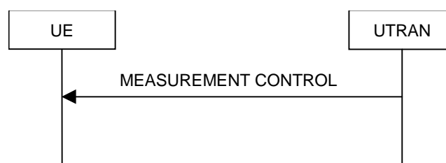
Figure 8.4.1-1: Measurement Control, normal case
