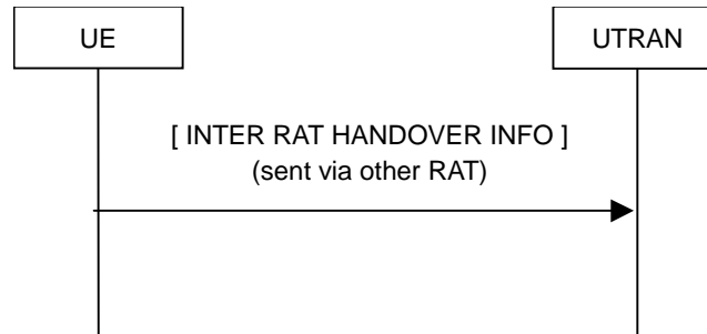
Figure 8.1.16-1: Inter RAT handover information transfer, normal flow
