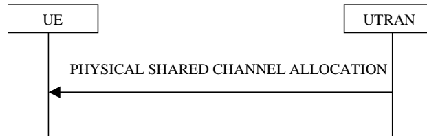
Figure 8.2.7-1: Physical Shared Channel Allocation
