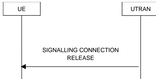
Figure 8.1.13-1: Signalling connection release procedure, normal case
