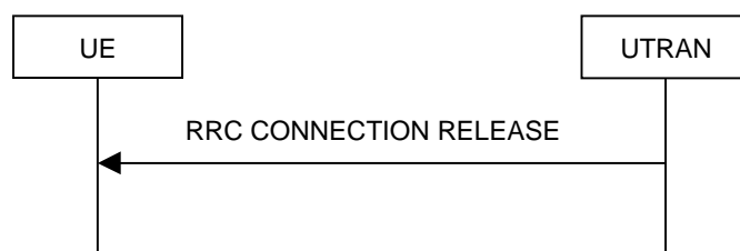
Figure 8.1.4-2: RRC Connection Release procedure on the CCCH
