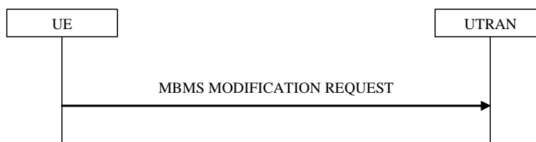
Figure 8.7.6-1: MBMS modification request, normal
