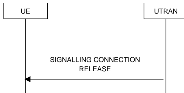
Figure 8.1.13-1: Signalling connection release procedure, normal case
