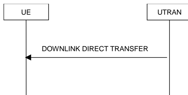
Figure 8.1.9-1: Downlink Direct transfer, normal flow
