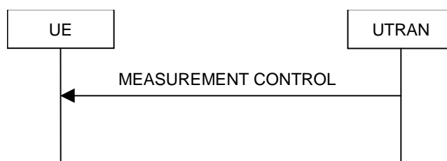
Figure 8.4.1-1: Measurement Control, normal case
