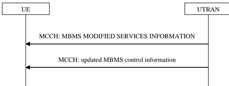
**Figure 8.7.3-1: MBMS notification on MCCH**
