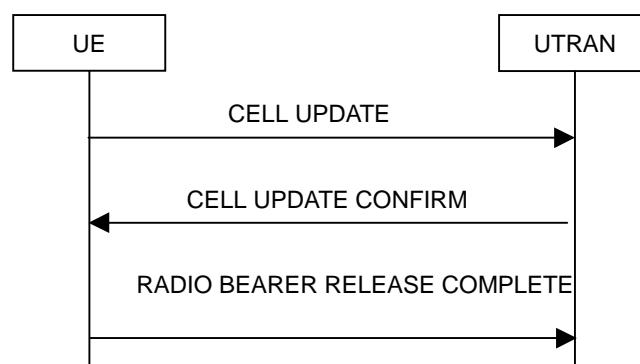
**Figure 8.3.1-5: Cell update procedure with radio bearer release**
