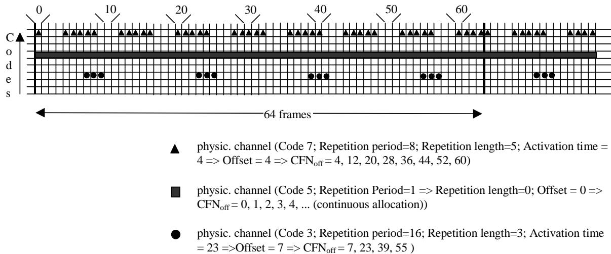
**Figure 8.6.6.16-1: Examples for frame allocations in TDD**
