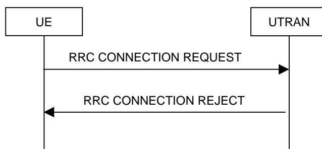
**Figure 8.1.3-2: RRC Connection Establishment, network rejects RRC connection**
