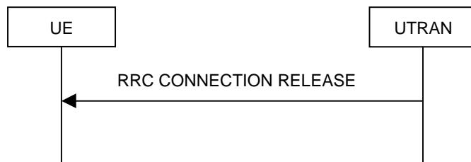
**Figure 8.1.4-2: RRC Connection Release procedure on the CCCH**
