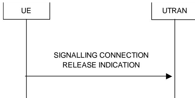
**Figure 8.1.14-1: Signalling connection release indication procedure, normal case**
