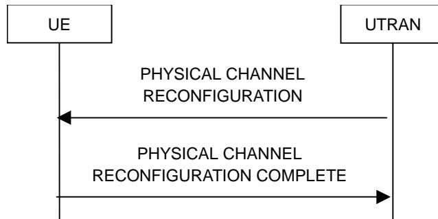
**Figure 8.2.2-9: Physical channel reconfiguration, normal flow**
