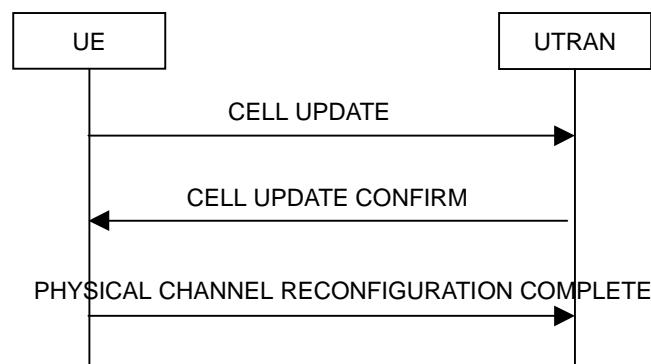
**Figure 8.3.1-3: Cell update procedure with physical channel reconfiguration**
