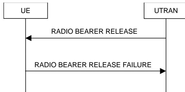
**Figure 8.2.2-6: Radio Bearer Release, failure case**
