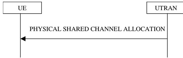
**Figure 8.2.7-1: Physical Shared Channel Allocation**
