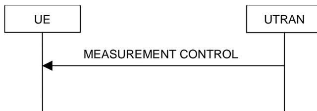
Figure 8.4.1-1: Measurement Control, normal case
