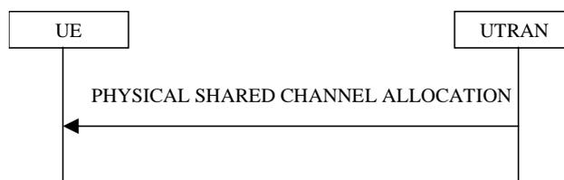
**Figure 8.2.7-1: Physical Shared Channel Allocation**
