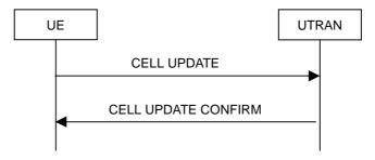
Figure 8.3.1-1: Cell update procedure, basic flow
