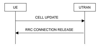
Figure 8.3.1-7: Cell update procedure, failure case
