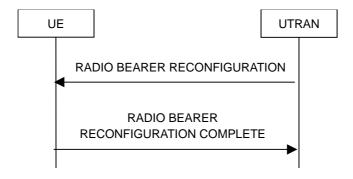
Figure 8.2.2-3: Radio bearer reconfiguration, normal flow
