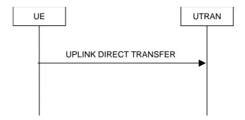
Figure 8.1.10-1: Uplink Direct transfer, normal flow
