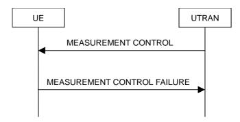
Figure 8.4.1-2: Measurement Control, failure case
