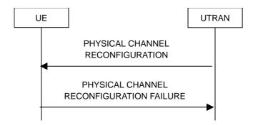
Figure 8.2.2-10: Physical channel reconfiguration, failure case
