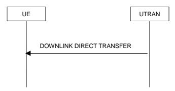
Figure 8.1.9-1: Downlink Direct transfer, normal flow
