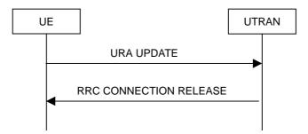
Figure 8.3.1-10: URA update procedure, failure case
