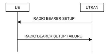
Figure 8.2.2-2: Radio Bearer Establishment, failure case
