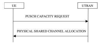
Figure 8.2.8-1: PUSCH Capacity request procedure
