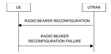
Figure 8.2.2-4: Radio bearer reconfiguration, failure case
