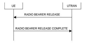
Figure 8.2.2-5: Radio Bearer Release, normal case
