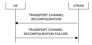
Figure 8.2.2-8: Transport channel reconfiguration, failure case
