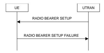
Figure 8.2.2-2: Radio Bearer Establishment, failure case
