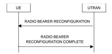
Figure 8.2.2-3: Radio bearer reconfiguration, normal flow
