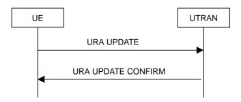
Figure 8.3.1-8: URA update procedure, basic flow
