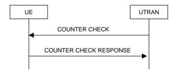
Figure 8.1.15-1: Counter check procedure
