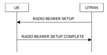
Figure 8.2.2-1: Radio Bearer Establishment, normal case
