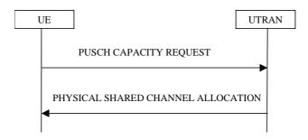
Figure 8.2.8-1: PUSCH Capacity request procedure
