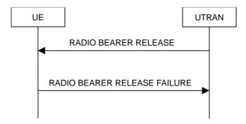
Figure 8.2.2-6: Radio Bearer Release, failure case
