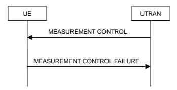
Figure 8.4.1-2: Measurement Control, failure case
