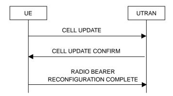
Figure 8.3.1-6: Cell update procedure with radio bearer reconfiguration
