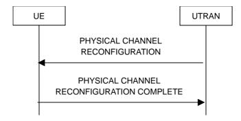
Figure 8.2.2-9: Physical channel reconfiguration, normal flow
