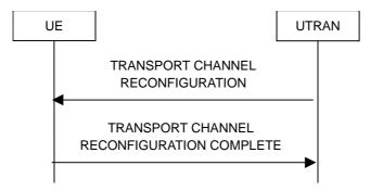
Figure 8.2.2-7: Transport channel reconfiguration, normal flow
