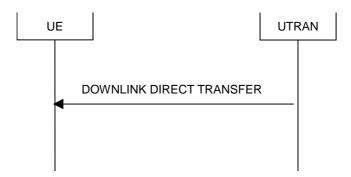
Figure 8.1.9-1: Downlink Direct transfer, normal flow
