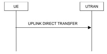
Figure 8.1.10-1: Uplink Direct transfer, normal flow
