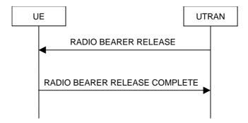
Figure 8.2.2-5: Radio Bearer Release, normal case
