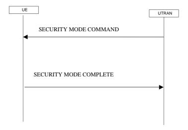
Figure 8.1.12-1: Security mode control procedure
