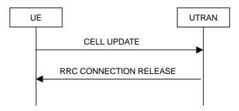
Figure 8.3.1-7: Cell update procedure, failure case
