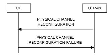
Figure 8.2.2-10: Physical channel reconfiguration, failure case
