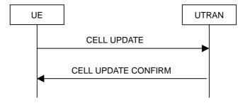
Figure 8.3.1-1: Cell update procedure, basic flow
