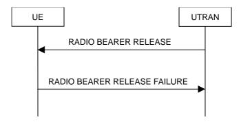
Figure 8.2.2-6: Radio Bearer Release, failure case
