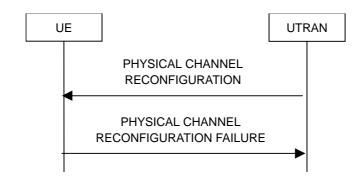
Figure 8.2.2-10: Physical channel reconfiguration, failure case
