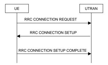
Figure 8.1.3-1: RRC Connection Establishment, network accepts RRC connection
