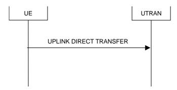
Figure 8.1.10-1: Uplink Direct transfer, normal flow
