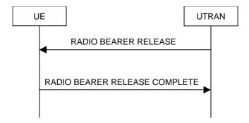
Figure 8.2.2-5: Radio Bearer Release, normal case
