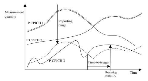
Figure 14.1.5.2-1: Time-to-trigger limits the amount of measurement reports
