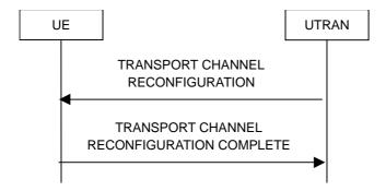
Figure 8.2.2-7: Transport channel reconfiguration, normal flow
