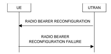
Figure 8.2.2-4: Radio bearer reconfiguration, failure case
