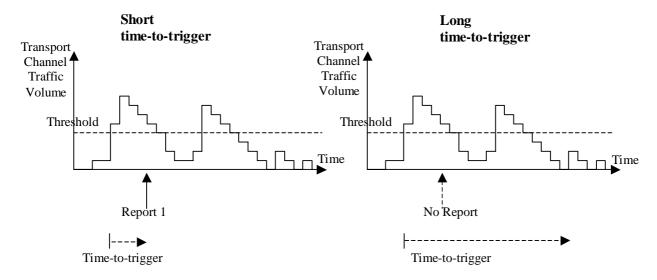
Figure 14.4.3.1-2: Time-to-trigger is used to achieve time hysteresis
