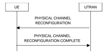
Figure 8.2.2-9: Physical channel reconfiguration, normal flow
