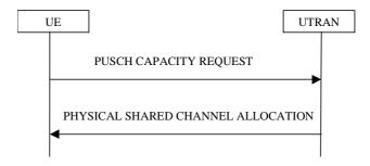
Figure 8.2.8-1: PUSCH Capacity request procedure
