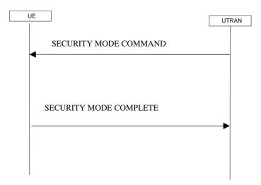
Figure 8.1.12-1: Security mode control procedure
