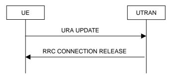
Figure 8.3.1-10: URA update procedure, failure case
