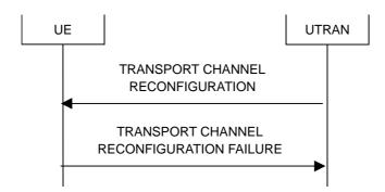
Figure 8.2.2-8: Transport channel reconfiguration, failure case
