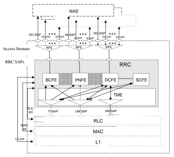
Figure 4.2-1: UE side model of RRC
