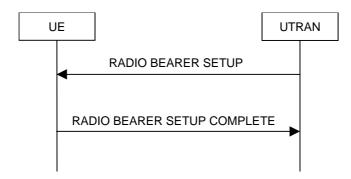
Figure 8.2.2-1: Radio Bearer Establishment, normal case
