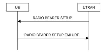
Figure 8.2.2-2: Radio Bearer Establishment, failure case
