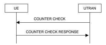
Figure 8.1.15-1: Counter check procedure
