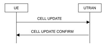
Figure 8.3.1-1: Cell update procedure, basic flow
