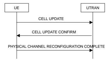
Figure 8.3.1-3: Cell update procedure with physical channel reconfiguration
