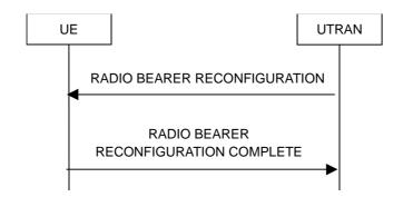
Figure 8.2.2-3: Radio bearer reconfiguration, normal flow
