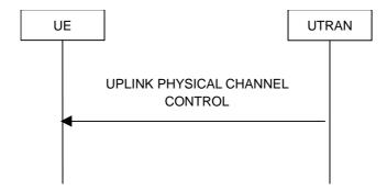
Figure 8.2.10-1: Uplink Physical Channel Control
