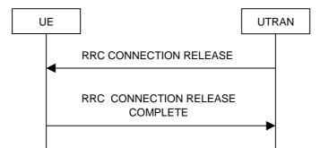
Figure 8.1.4-1: RRC Connection Release procedure on the DCCH
