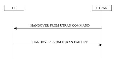
Figure 8.3.7-2: Inter-RAT handover from UTRAN, failure case
