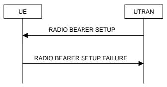
Figure 8.2.2-2: Radio Bearer Establishment, failure case
