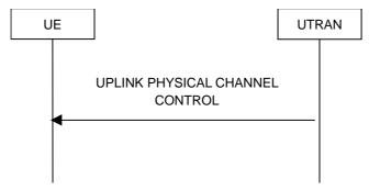
Figure 8.2.10-1: Uplink Physical Channel Control
