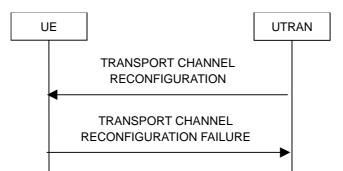
Figure 8.2.2-8: Transport channel reconfiguration, failure case
