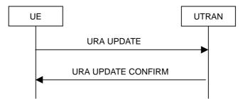
Figure 8.3.1-8: URA update procedure, basic flow
