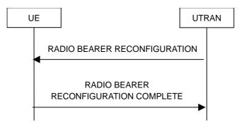
Figure 8.2.2-3: Radio bearer reconfiguration, normal flow
