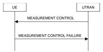
Figure 8.4.1-2: Measurement Control, failure case
