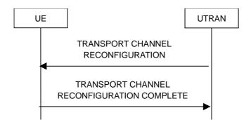
Figure 8.2.2-7: Transport channel reconfiguration, normal flow
