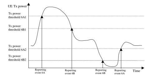
Figure 14.6.2.2-1: Event-triggered measurement reports when the UE Tx power becomes larger or less than absolute thresholds
