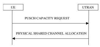
Figure 8.2.8-1: PUSCH Capacity request procedure
