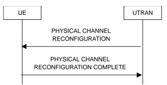
Figure 8.2.2-9: Physical channel reconfiguration, normal flow
