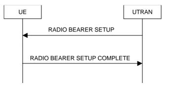
Figure 8.2.2-1: Radio Bearer Establishment, normal case
