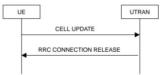
Figure 8.3.1-7: Cell update procedure, failure case
