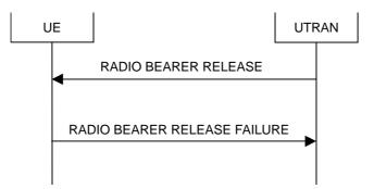
Figure 8.2.2-6: Radio Bearer Release, failure case
