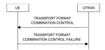
Figure 8.2.5-2: Transport format combination control, failure case
