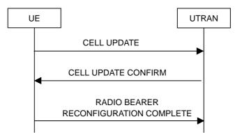
Figure 8.3.1-6: Cell update procedure with radio bearer reconfiguration
