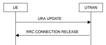
Figure 8.3.1-10: URA update procedure, failure case
