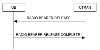
Figure 8.2.2-5: Radio Bearer Release, normal case
