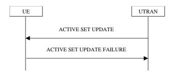
Figure 8.3.4-2: Active Set Update procedure, failure case
