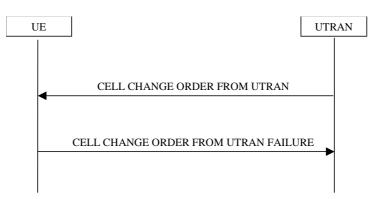
Figure 8.3.11-2: Inter-RAT cell change order from UTRAN, failure case
