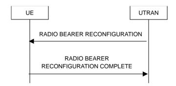
Figure 8.2.2-3: Radio bearer reconfiguration, normal flow
