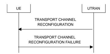
Figure 8.2.2-8: Transport channel reconfiguration, failure case
