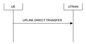
Figure 8.1.10-1: Uplink Direct transfer, normal flow
