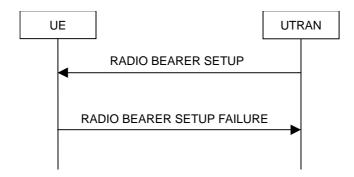
Figure 8.2.2-2: Radio Bearer Establishment, failure case
