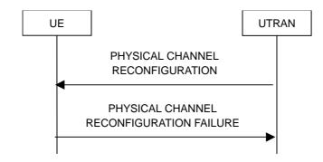
Figure 8.2.2-10: Physical channel reconfiguration, failure case
