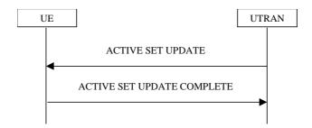
Figure 8.3.4-1: Active Set Update procedure, successful case
