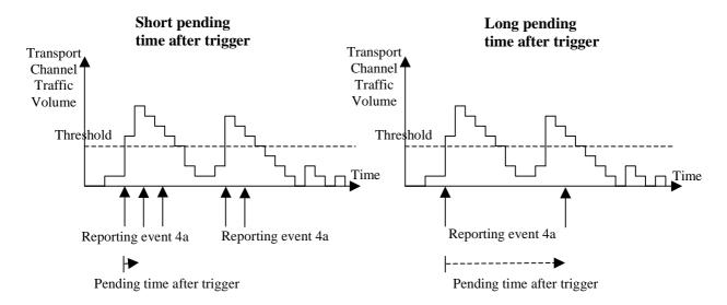
Figure 14.4.3.1-1: Pending time after trigger limits the amount of consecutive measurement reports
