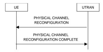
Figure 8.2.2-9: Physical channel reconfiguration, normal flow
