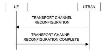
Figure 8.2.2-7: Transport channel reconfiguration, normal flow
