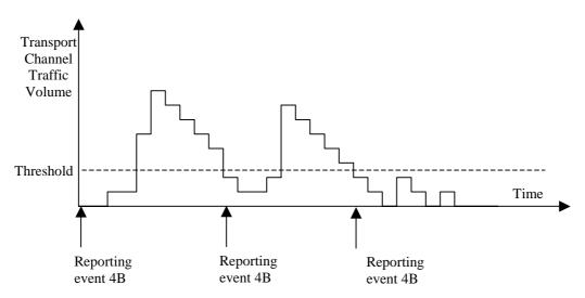
Figure 14.4.2.1-2: Event triggered report when Transport Channel Traffic Volume becomes smaller than certain threshold
