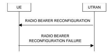
Figure 8.2.2-4: Radio bearer reconfiguration, failure case
