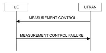
Figure 8.4.1-2: Measurement Control, failure case
