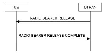
Figure 8.2.2-5: Radio Bearer Release, normal case
