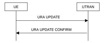
Figure 8.3.1-8: URA update procedure, basic flow
