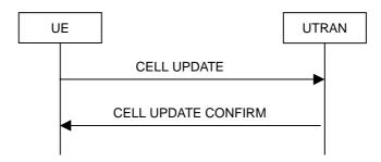
Figure 8.3.1-1: Cell update procedure, basic flow
