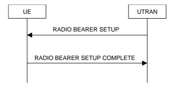
Figure 8.2.2-1: Radio Bearer Establishment, normal case
