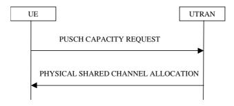
Figure 8.2.8-1: PUSCH Capacity request procedure
