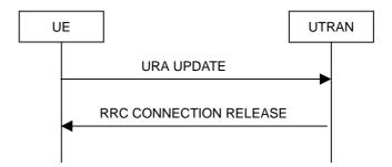
Figure 8.3.1-10: URA update procedure, failure case
