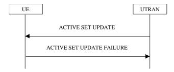
Figure 51: Active Set Update procedure, failure case
