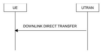
Figure 15: Downlink Direct transfer, normal flow
