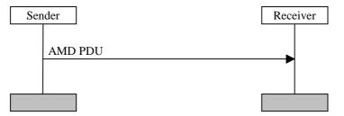
Figure 11.3: Acknowledged mode data transfer procedure
