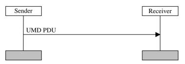
Figure 11.2: Unacknowledged mode data transfer procedure
