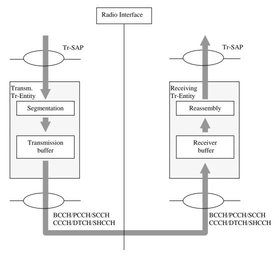
Figure 4.2: Model of two transparent mode peer entities
