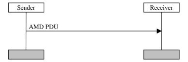
Figure 11.3: Acknowledged mode data transfer procedure
