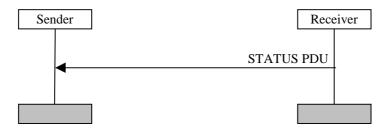
Figure 11.5: STATUS PDU transfer procedure
