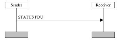
Figure 11.6: SDU discard with explicit signalling
