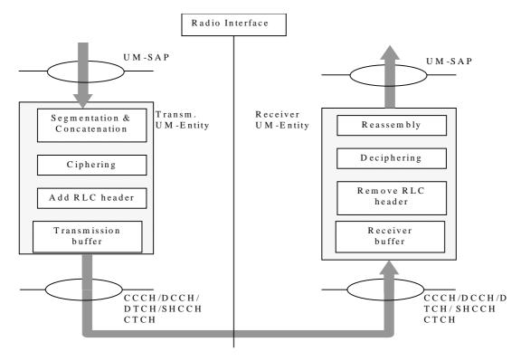
Figure 4.3: Model of two unacknowledged mode peer entities
