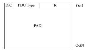
Figure 9.6: RESET, RESET ACK PDU
