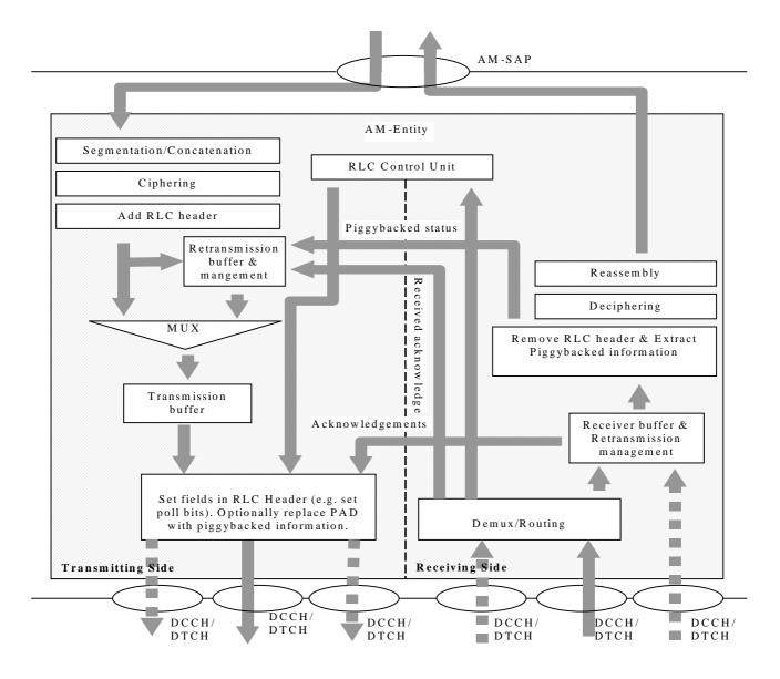
Figure 4.4: Model of a acknowledged mode entity
