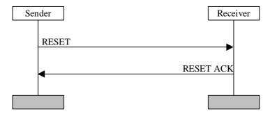
Figure 11.4: RLC reset procedure
