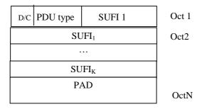
Figure 9.4: Status Information Control PDU (STATUS PDU)
