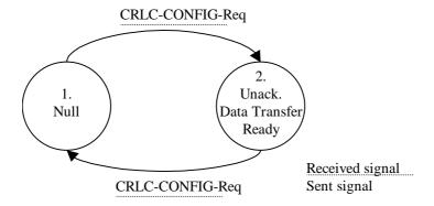
Figure 9.17: The state model for unacknowledged mode entities
