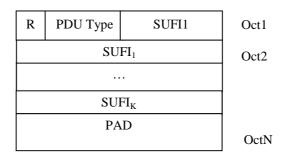
Figure 9.5: Piggybacked STATUS PDU
