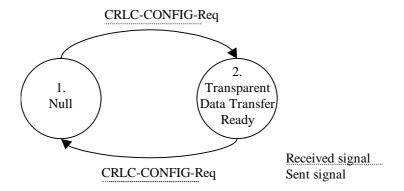
Figure 9.16: The state model for transparent mode entities
