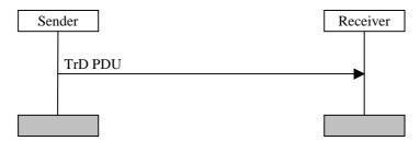
Figure 11.1: Transparent mode data transfer procedure
