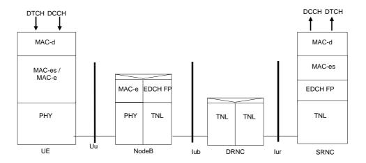
Figure 6.1-1: Protocol Architecture of E-DCH
