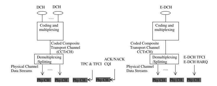
Figure 6.3.1-1: Model of the UE's Uplink physical layer
