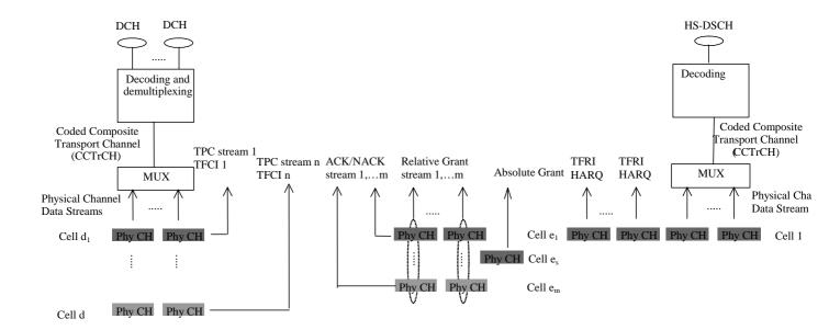
Figure 6.3.2-1: Model of the UE's Downlink physical layer. HS-DSCH serving cell is cell 1 in this figure
