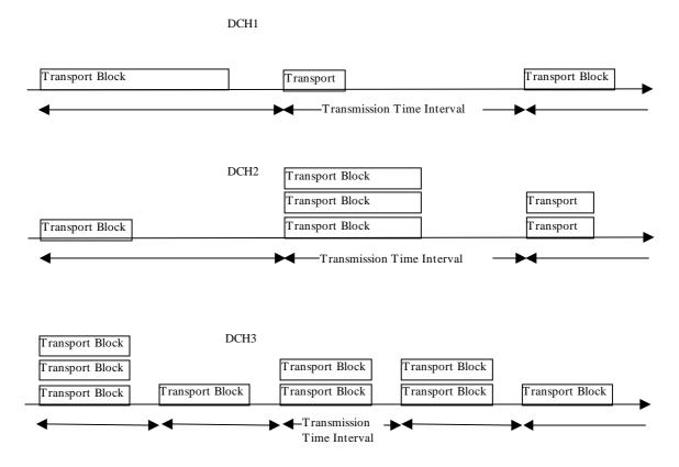
Figure 6: Exchange of data between MAC and L1
