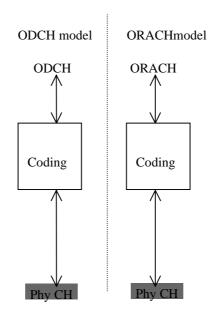
Figure 5: Model of the UE's physical lay-r - relay link TDD mode.
