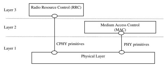
Figure 1: Interfaces with the Physical Layer
