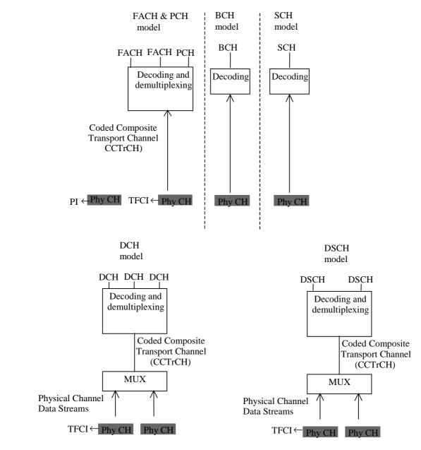
Figure 4: Model of the UE's physical layer - downlink TDD mode
