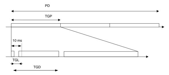
Figure 7: Illustration of compressed mode pattern parameters.
