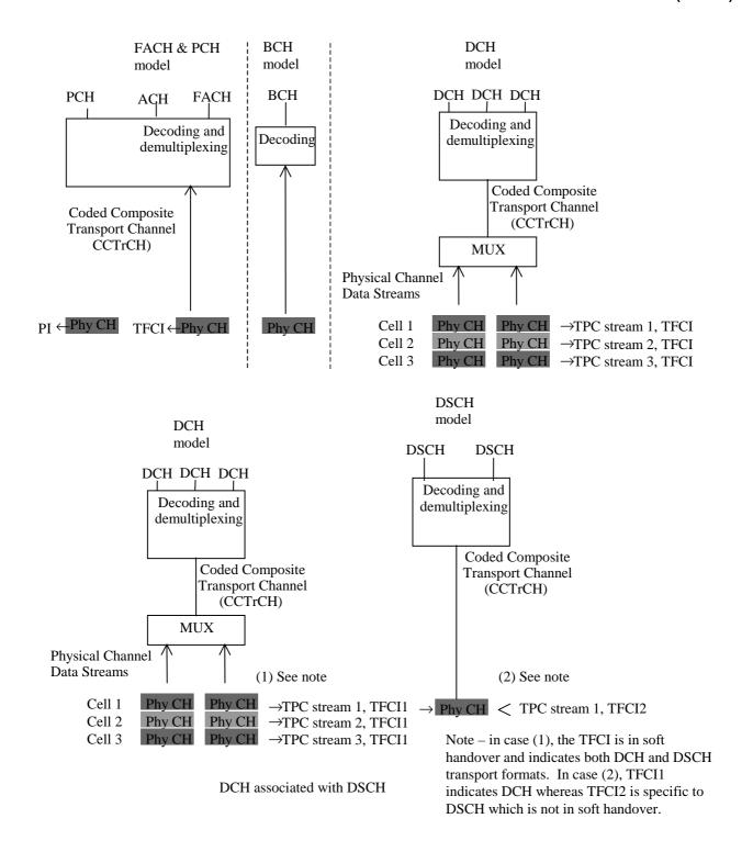
Figure 3: Model of the UE's physical layer – downlink FDD mode
