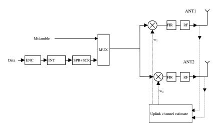
Figure 1: Downlink transmitter structure to support Transmit Diversity for PDSCH, DPCH, HS-SCCH, and HS-PDSCH transmission (UTRAN Access Point)
