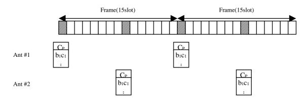
Figure 3: Antenna Switching Pattern (Case 2)
