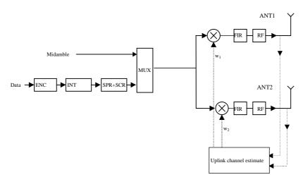
Figure 8: Downlink transmitter structure to support Transmit Diversity for DPCH, PDSCH, HS-SCCH, and HS-PDSCH transmission (UTRAN Access Point) in 1.28 Mcps TDD
