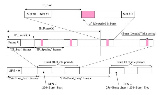
Figure 5 below illustrates the idle periods for the burst mode case, if the IP\_P-CCPCH parameter is set to 0.
