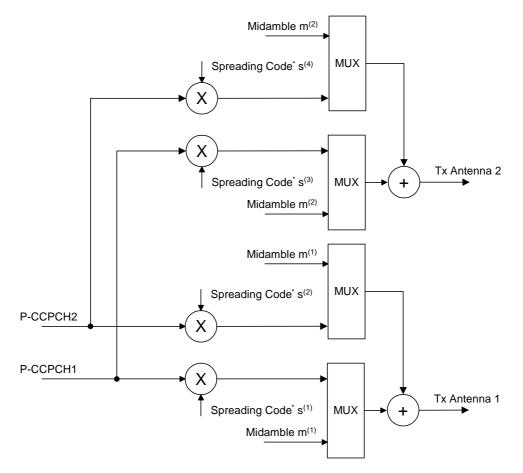
\* Spreading by s<sup>(k)</sup> means channelisation by c<sup>(k)</sup> and cell specific scrambling
