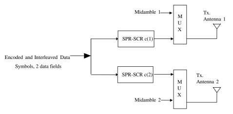
Figure 4: Block Diagram of the transmitter SCTD
