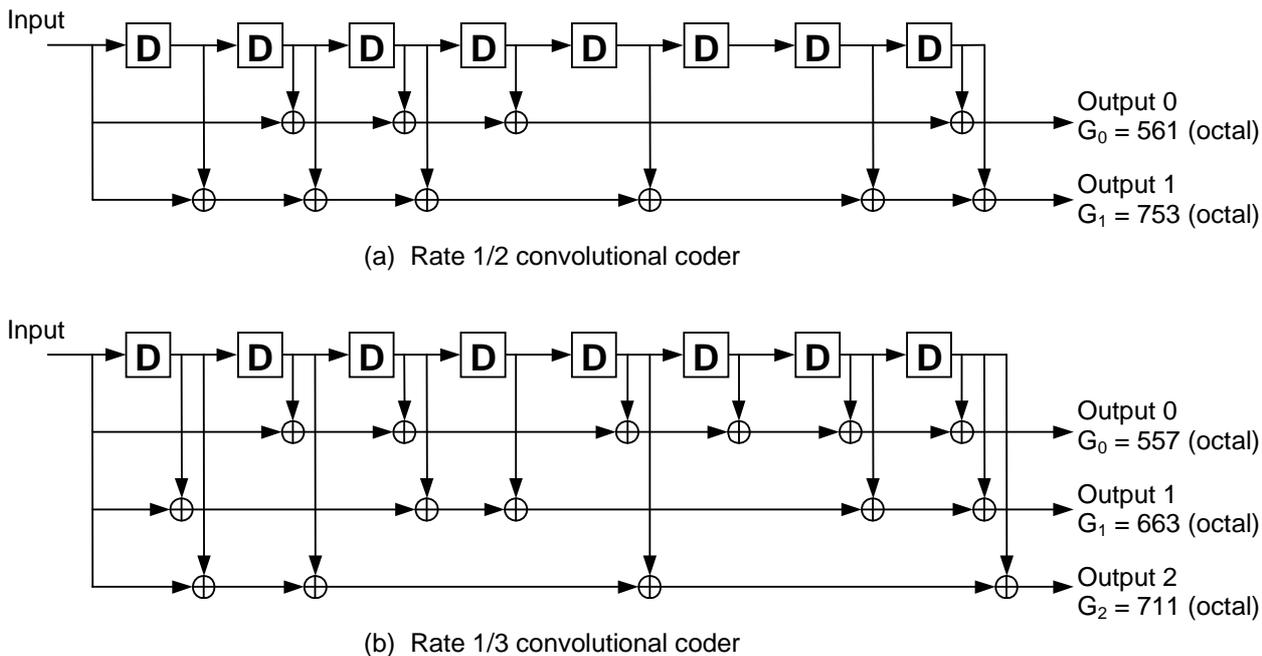
Figure 2: Rate 1/2 and rate 1/3 convolutional coders
