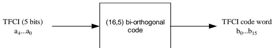
Figure 7: Channel coding of short length TFCI bits
