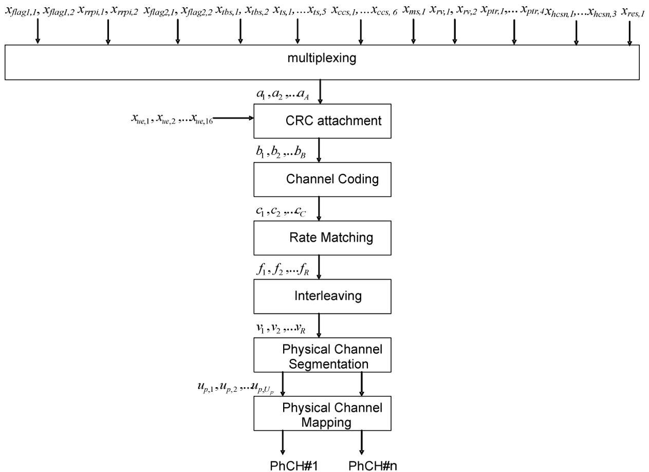
Figure 19B: Coding and Multiplexing for HS-SCCH type 3
