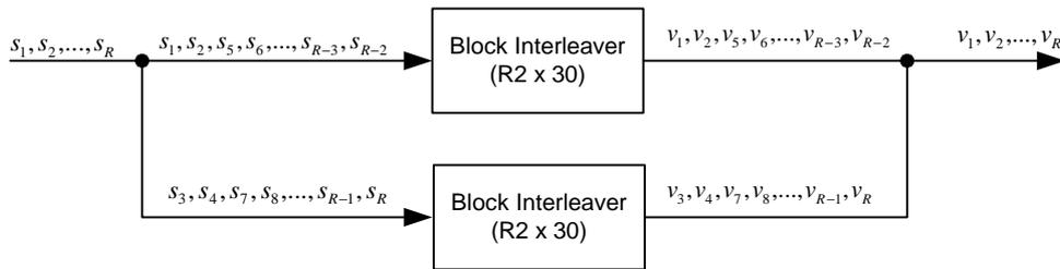
Figure 18: Interleaver structure for HS-DSCH with 16-QAM modulation
