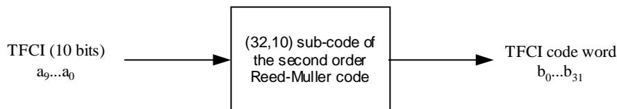
Figure 6: Channel coding of the TFCI bits
